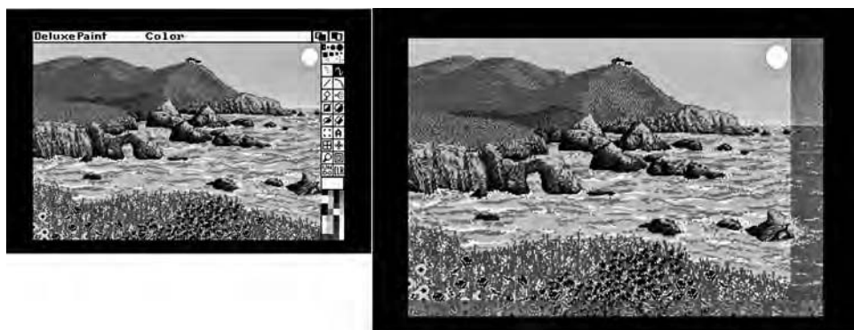
3.3 On the left is the Deluxe Paint screen as the user sees it; on the right is the master copy of the image being worked on, which is stored elsewhere in memory. Those parts of the master copy that are darkened are not copied into the screen that the user sees but nevertheless are still part of the image.
