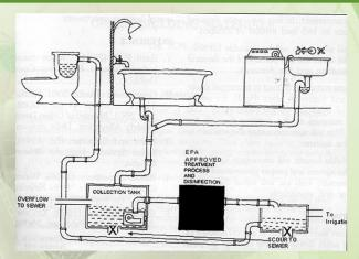
The dual plumbing system in which used water can be recycled for flushing of toilets and drain water can be used for irrigation and gardening purposes.
