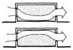
Louvres can direct airflow upward or downward.
