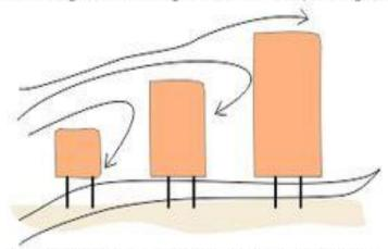
if a site has multiple buildings, they should be arranged in ascending order of their heights and be built on stilts to allow ventilation
