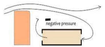
Taller forms in the wind direction of prevailing wind can alter the wind movement pattern for low lying buildings behind them
