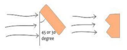
Place buildings at a 30 or 45 degree angle to the direction of wind for enhanced ventilation. Form can be staggered in the wind facing direction also to achieve the same result.
