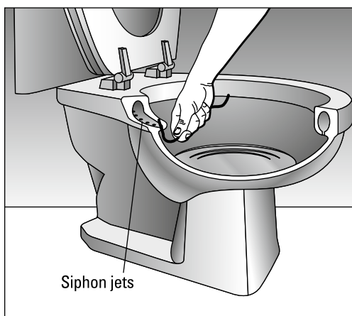
FIGURE 8-1: Clearing clogged siphon jets.
