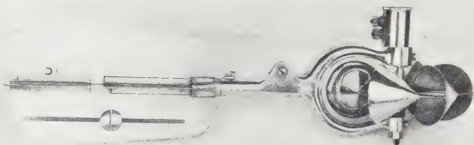
FIG. 2. Price-type current meter (U.S. Geological Survey).
