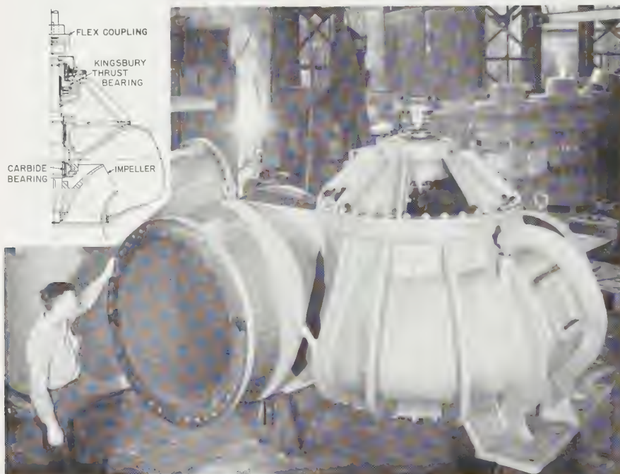
FIG. 49. Mixed-flow volute pump rated 70,000 gpm, 34.3-ft total head, 349 rpm, for a municipal sewage-treatment plant. Sketch shows one of bearing arrangements used in pumps of this design. ( Baldwin-Lima-Hamilton Corp. )
