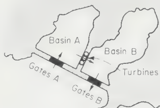
FIG. 7. Typical layout for two-basin scheme for continuous power generation or peaking power.
