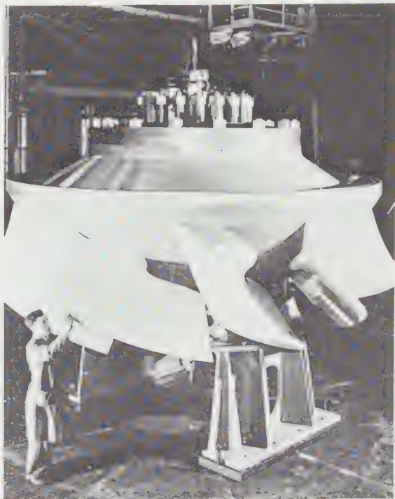
FIG. 71b. Shop assembly of diagonal-flow adjustable-blade Deriaz-type impeller runner of pump-turbine rated 108,500 hp, 243-ft head, 150 rpm for Valdecanas plant of Hidro-electrica Espanola S.A., Spain. (Three units by English Electric Company Ltd.)
