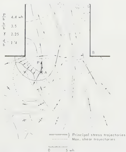
FIG. 7. Principal stresses and their trajectories for case illustrated in Fig. 5.
