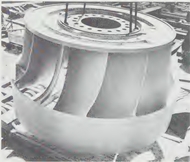
FIG. 6. Francis-type runner for one of the Garrison Dam power-plant turbines rated 90,000-hp, 150-ft net head, 90 rpm. Runner is one of the largest cast in one piece in the United States. Outside diameter 223.5 in.; weight 150,000 lb. ( Baldwin-Lima-Hamilton Corp. )
