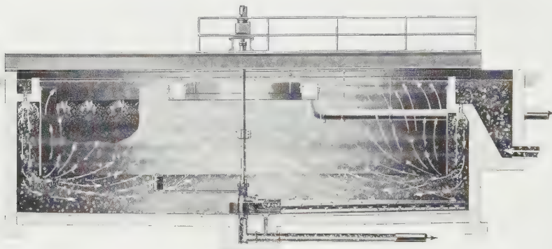
FIG. 19. Density currents and flow patterns in final tank. ( Chain Belt Co. )
