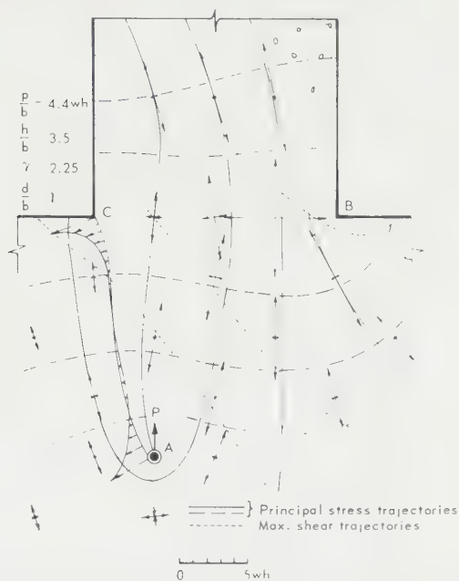
FIG. 6. Principal stresses and their trajectories for case illustrated in Fig. 4.
