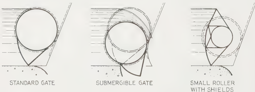
FIG. 12. Types of rolling gates.
