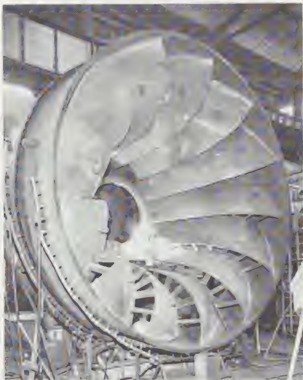
FIG. 5. Francis-type runner for one of the turbines rated 204,000-hp, 179-ft net head, 100 rpm for the Smith Mountain Dam powerhouse. Runner fabricated by welding weighs 285,000 lb and has outside diameter exceeding 246 in., requiring splitting upon completion into halves for shipping. ( Baldwin-Lima-Hamilton Corp. )
