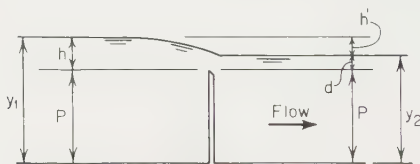
FIG. 57. Sharp-crested weir with submerged two-dimensional overflow.
