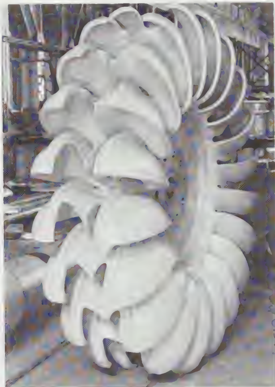
FIG. 3. Impulse turbine runner (Pelton type) with buckets cast integrally with the hub. ( Allis-Chalmers Mfg. Co. )
