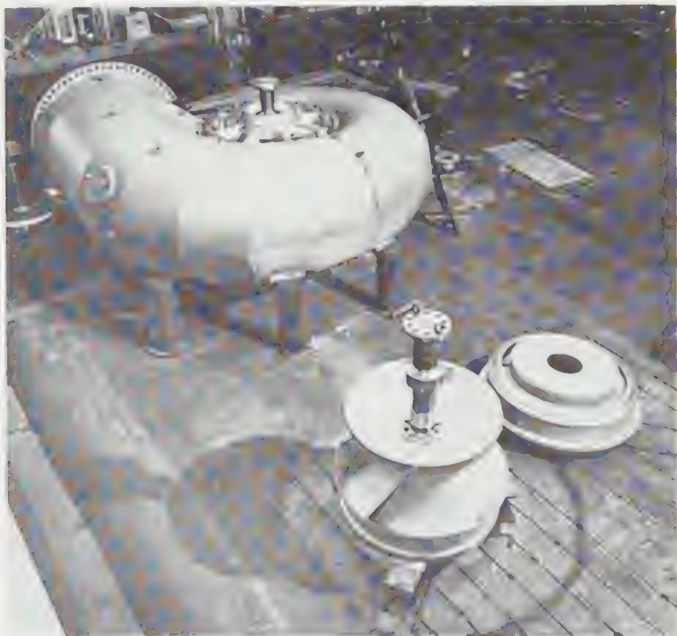
FIG. 53. Shop assembly of one of two condenser circulating pumps for Joliet Station of Commonwealth Edison Company. Impeller and top plate of other unit in foreground. Pump rating: 230,000 gpm at 30-ft head, 212 rpm. ( Allis-Chalmers Mfg. Co. )
