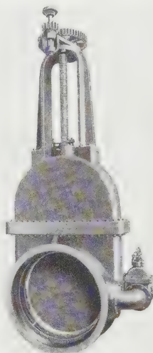
FIG. 14b. Outside-screw-and-yoke-type cast-iron gate valve with spur gears and bypass. ( Rensselaer. )
