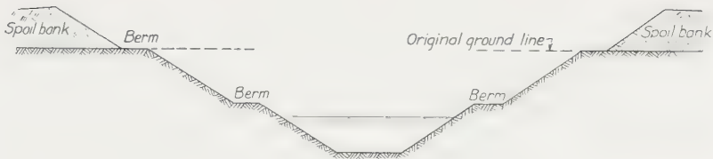
FIG. 7. Typical deep-cut canal section.
