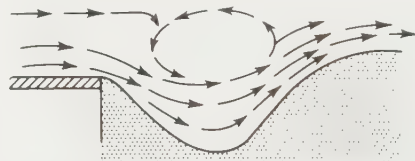
FIG. 6. Undesirable ground-roller pattern— without end sill.
