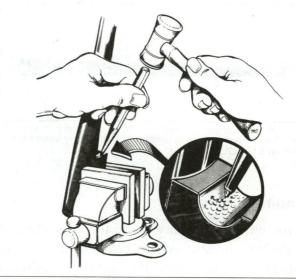
Figure 3-4: Peening barrel lug to tighten barrel/receiver fit on single-shot shotgun.
