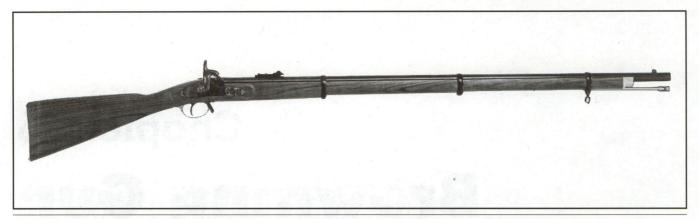
Figure 16-2: Almost all muzzleloading firearms manufactured prior to about 1865 were browned rather than blued.
