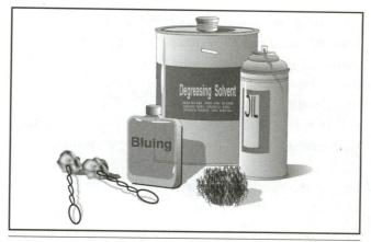
Figure 15-2: Basic items required for cold bluing: cleaning solution, steel wool, applicators, oil, and the cold (instant) bluing solution.
