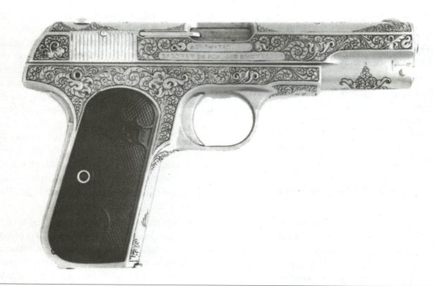
Figure 17-5: This .32 ACP Colt semiautomatic pistol has been highly engraved besides being nickel plated.
