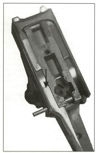
Figure 11-2: Sears on many double shotguns — especially some of the inexpensive foreign models — were often made of relatively soft metal, which eventually wore and usually resulted in both barrels firing simultaneously. One solution to this problem is to cut off the tip of the sear, and silver solder another piece of good hardened steel in its place.
