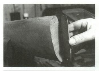
Figure 21-14: Saw cuts must be smoothed with wood rasps and files prior to installing the plate, especially if a skeleton-type plate is to be put on the gunstock.
