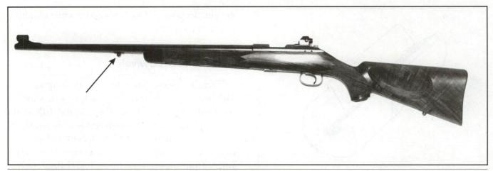
Figure 21-10: Swivel stud soldered (sweated) on the bottom of the barrel.
