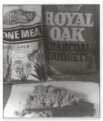
Figure 12-1: The main ingredients for a simple casehardening operation are bone meal, charcoal, and leather.
