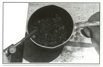
Figure 12-2: Once mixed, the ingredients should be charred and pulverized before packing the part in them.
