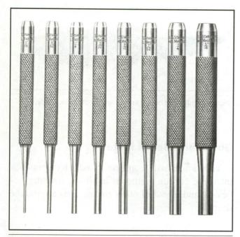
Figure 3-3: Pin punches are necessary to disassemble practically any gun that has ever been manufactured.
