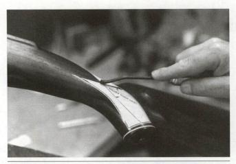
Figure 19-10: Use a single-line cutter to cut out the border and guidelines of the checkering pattern, using the groove cut with the sharp knife as a guide.
