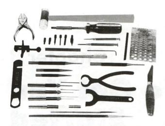
Figure 3-1: Brownells Assembly/Disassembly Tool Kit.
