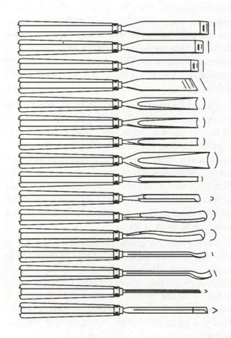
Figure 18-16: Sizing and sweeps of typical wood carving tools.
