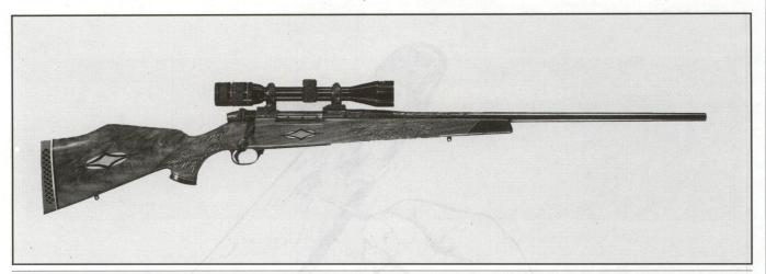
Figure 20-5: Sometimes it is best to use inlays in a gunstock to cover gouges rather than trying to splice a piece of matching wood.
