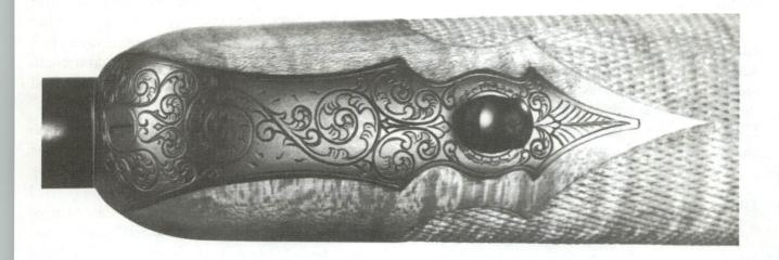
Figure 18-20: You must also inlet any flush-mounted stock furniture like this fancy combination forend tip and sling swivel.
