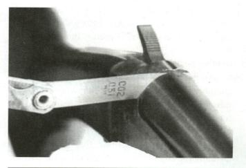
Figure 10-3: Feeler gauge being used to measure the gap between the barrel and standing breech.
