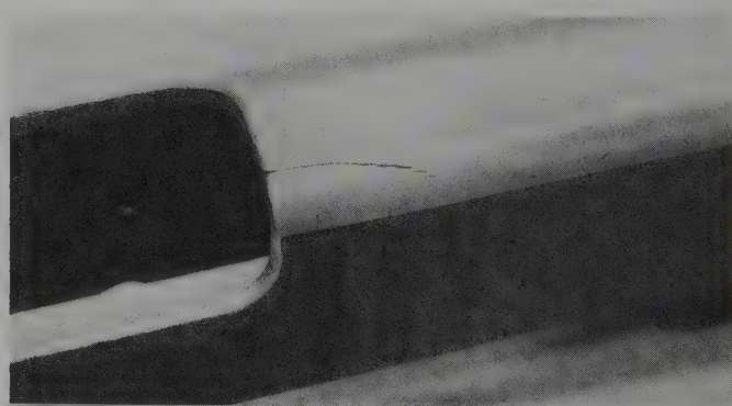
If you do not brace your hand when using a hand-held grinder, the stone may slip. If you are lucky, you may only mar your handgun, as on this 1911 slide. You may hurt yourself.
