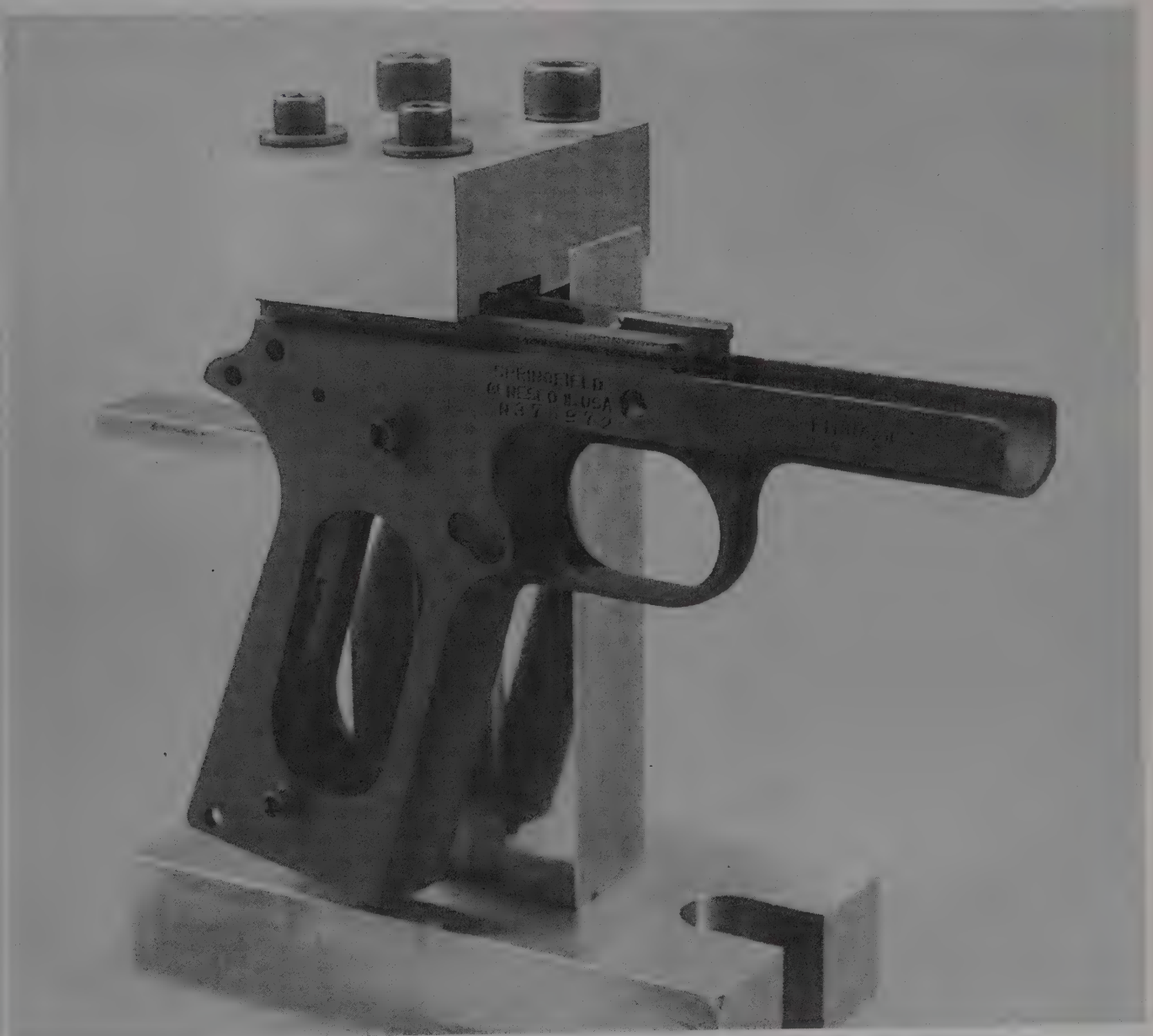
The Cominolli fixture is so sturdy I'm not sure you could hurt it running it over with a truck. The frame is held here for one of the ramped barrel cuts.
