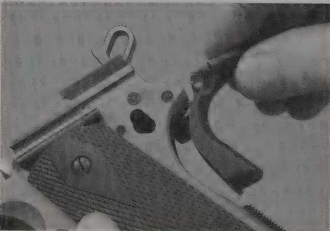
With the mainspring housing slightly lowered, lift the grip safety out of the frame.
