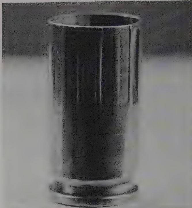
This case came out of an H-K MP-5 sub-machine gun. The flutes that aid extraction also crinkle the cases. This case can be reloaded once again, and then it will expire.
