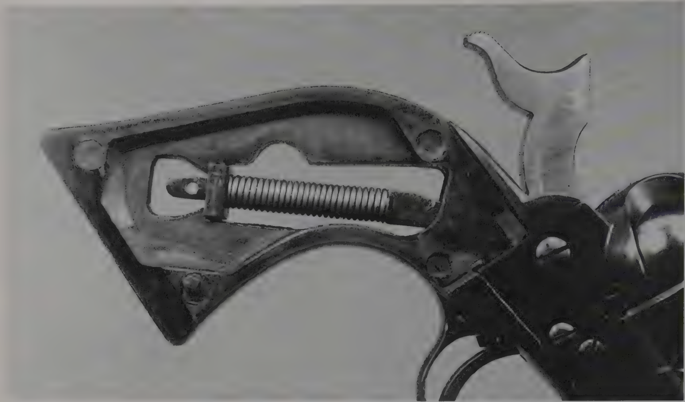
The Ruger re-design of the single-action revolver replaced the flat mainspring with a coil spring that works over a shaft.
