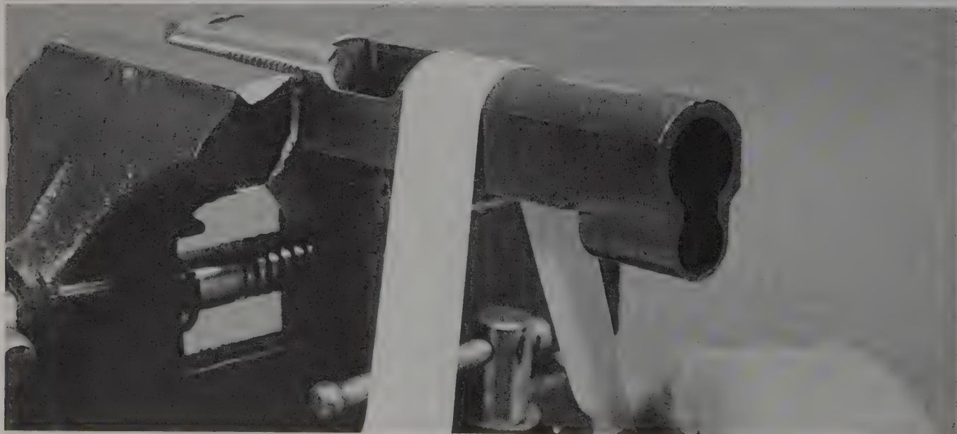
Holding the cloth down on the sides sands the entire radius of this slide.
