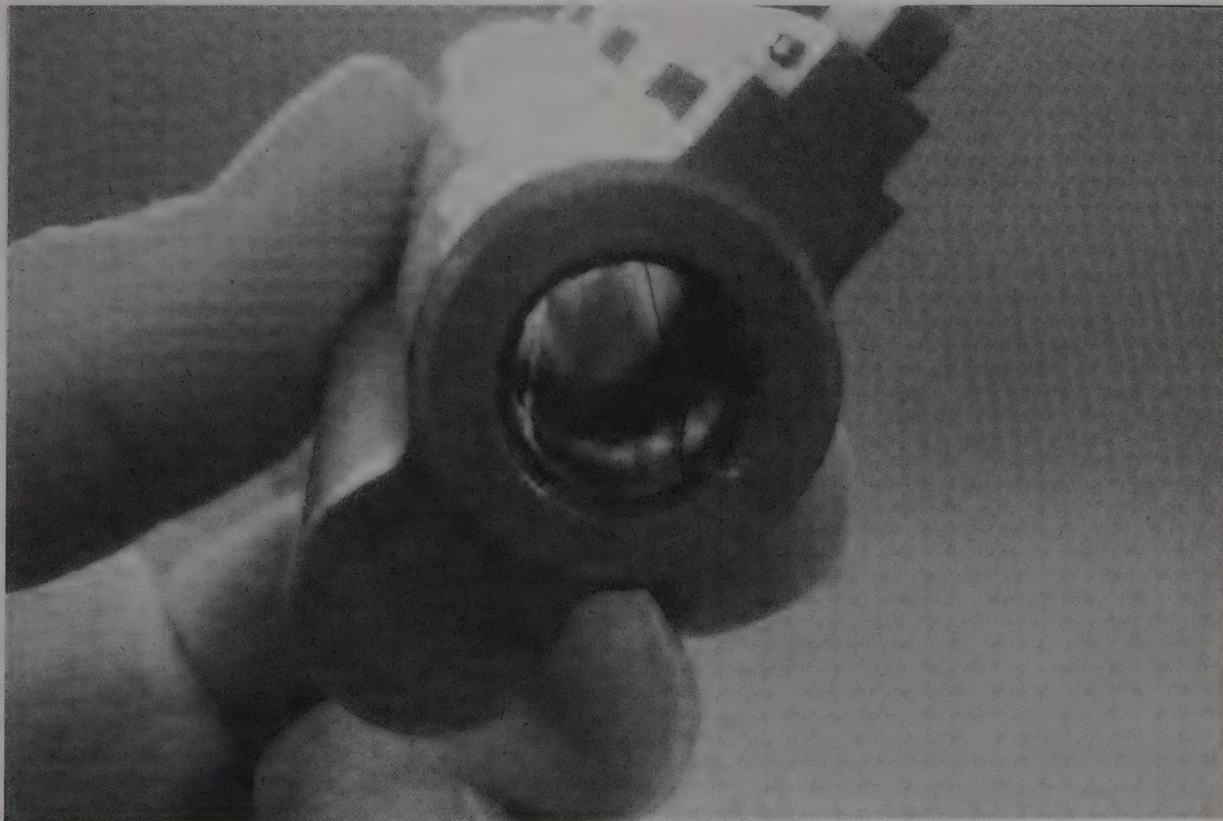
This ring is right near the muzzle, and the barrel might be salvaged if it is shortened.
