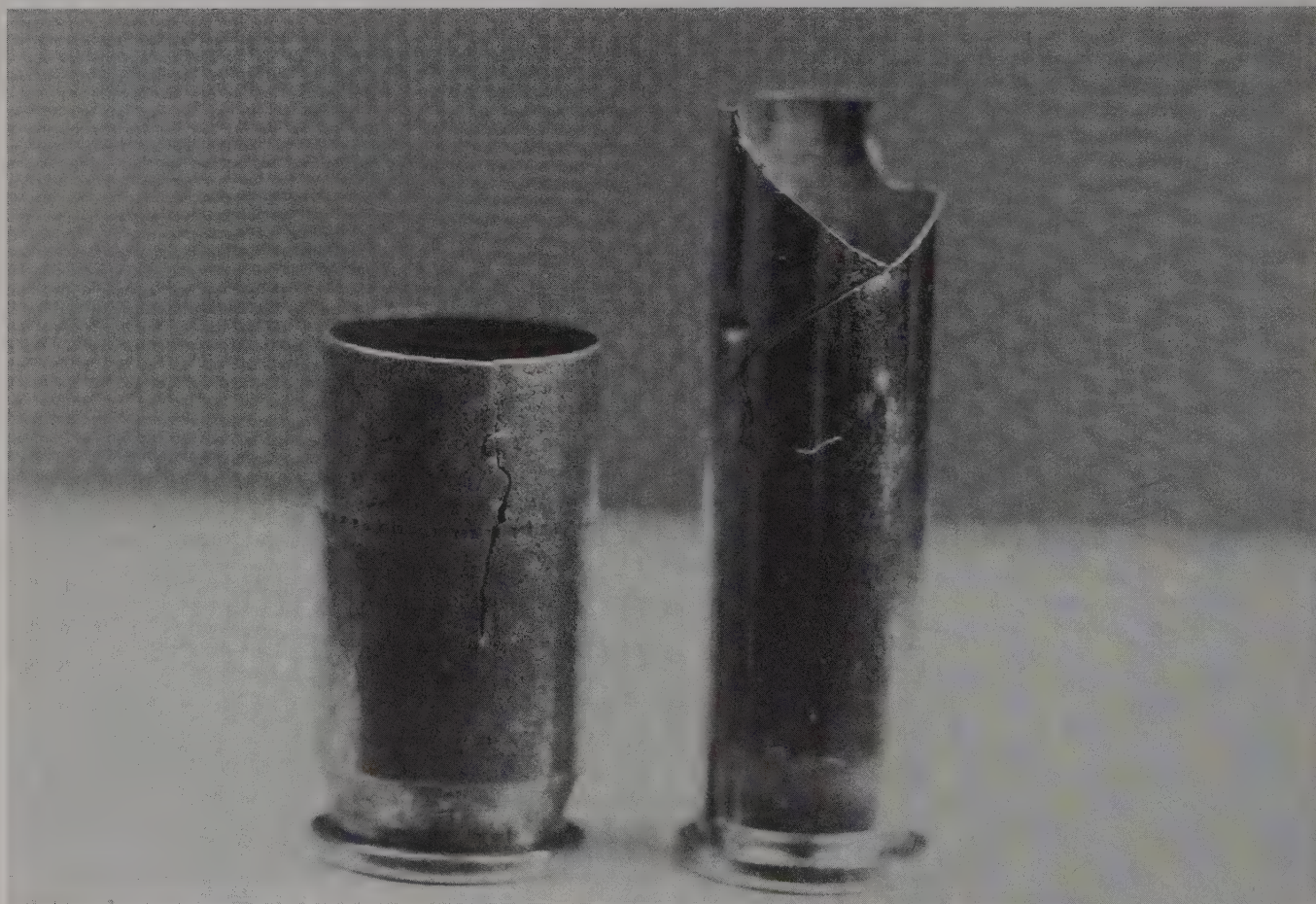
Cracked or broken cases will prevent your handgun from working properly.
