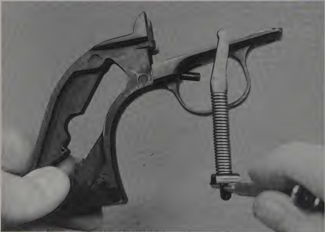
After cocking the mainspring, place a punch or small screwdriver through the hole in the shaft. Remove the five screws, and the grip frame comes off in one piece. The plunger in the trigger guard is the trigger return spring and plunger.
