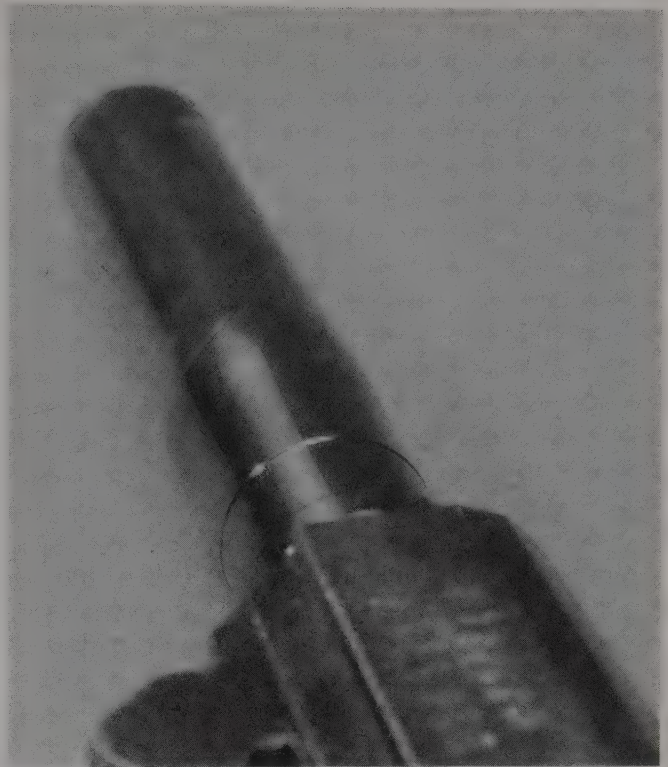
Seen at an angle, the bulge in this barrel is obvious.
