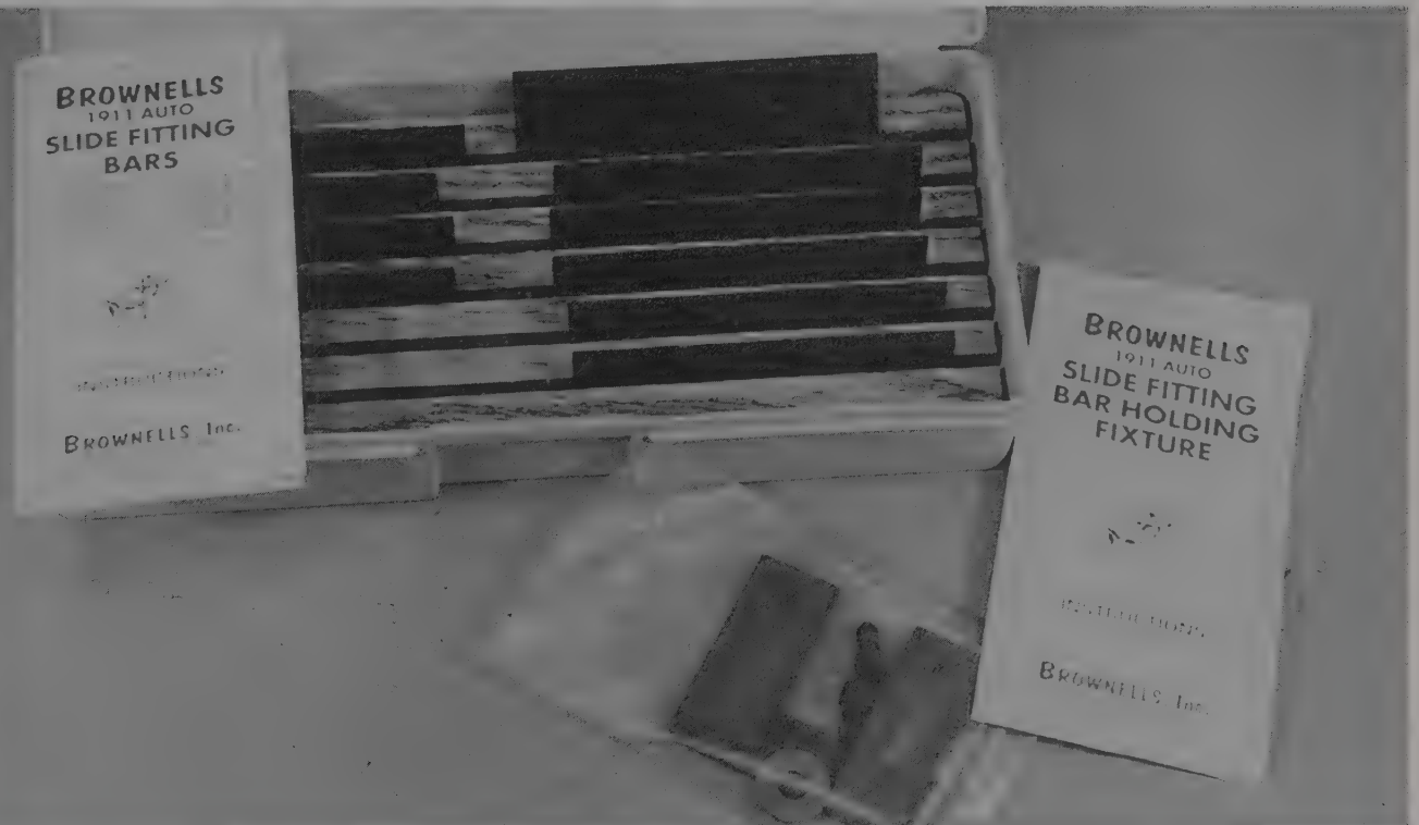
Here are the forming rails and the holding fixture. With the holding fixture, you can peen the rails without a vise or vise-holding plates.
