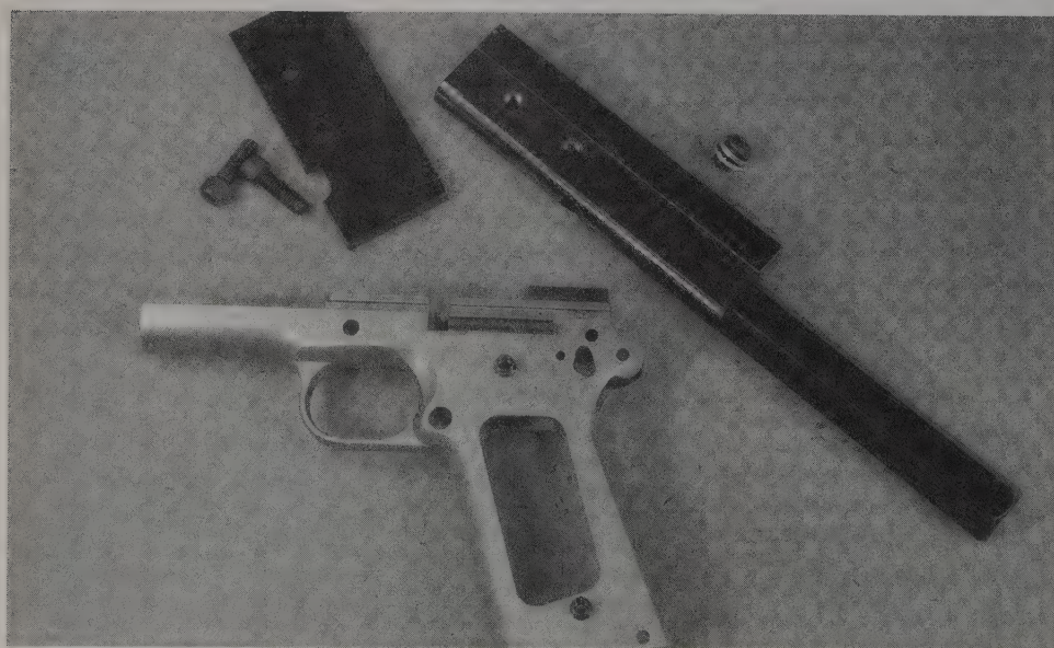
The Wilson frame holder is a solid piece of steel that allows you to hold your frame in the vise without damage. You can also make your own frame holder.
