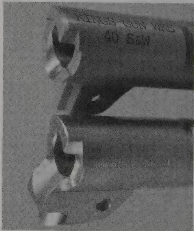
Both these barrels are in .40 S&W, but the Infinity barrel is the choice of many competitors because of the ramp. If you are not going to push your loads to (or past) the red line, the Kings barrel will be accurate, dependable and give a long service life.
