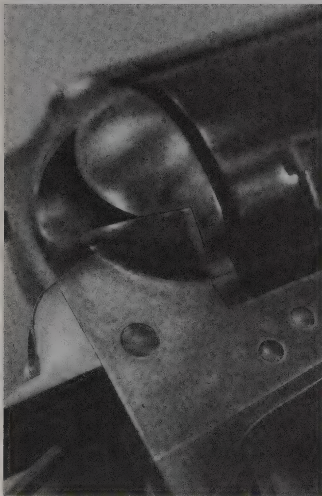
Color case-hardening is an old method of both protecting the surface and hardening the iron. While attractive, it doesn't do either very well.
