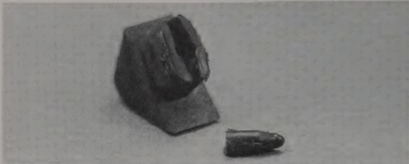
The Glock front sight and its wedge.
