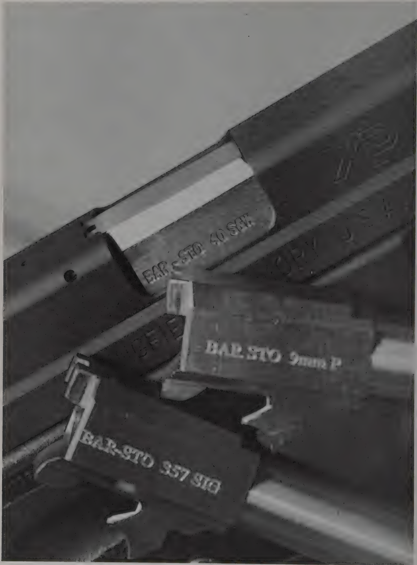
If you start with an XD or XD ® in 40, you can have extra barrels fitted for .357 SIG and 9mm.
