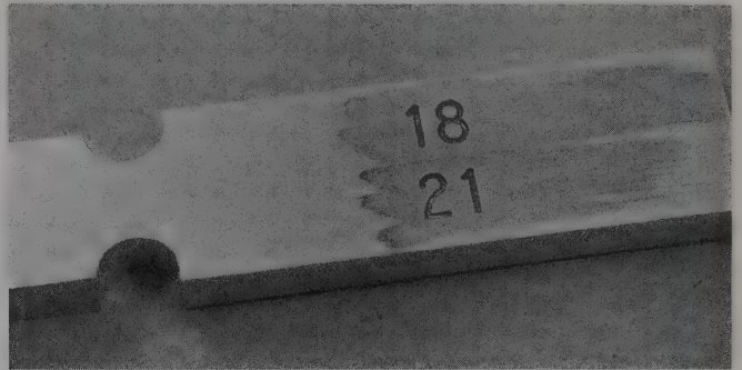
The EGW hood gauge makes a tough task easy: measuring the distance from breechface to front locking lugs on the slide.
