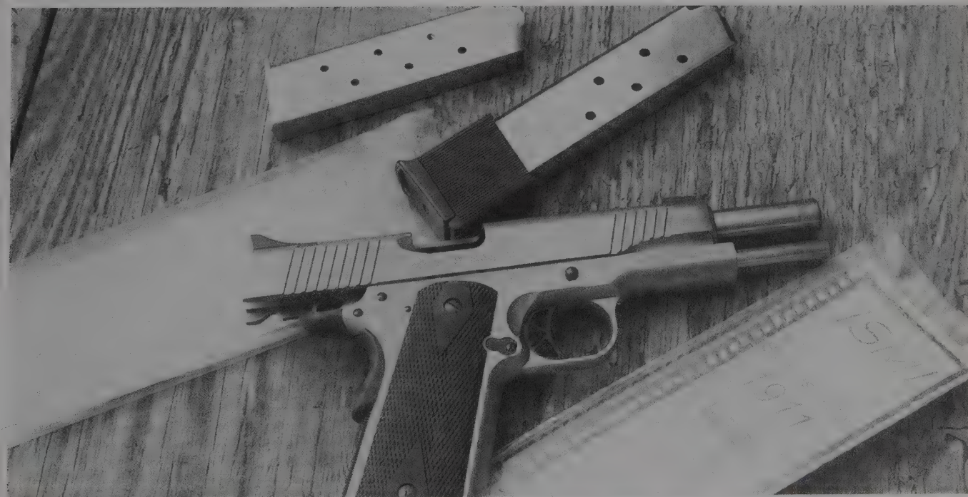
The Kimber at the range, ready to consume 1,400 rounds of ammunition, testing the springs. The pistol gobbled all that ammo without a problem.
