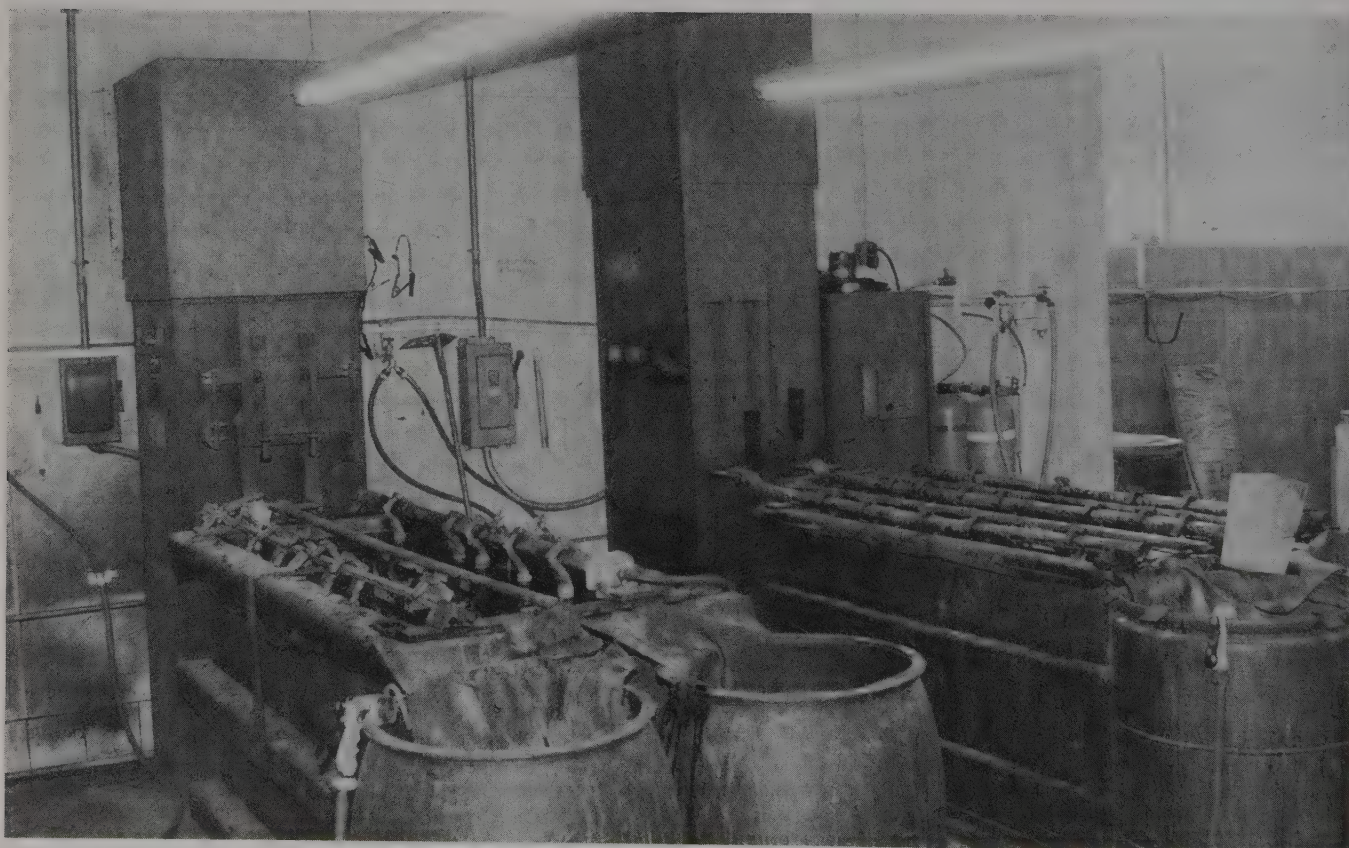
Firearms refinishing requires tanks, chemicals and lots of ventilation. This plating room at Accurate Plating uses the natural breezes of the Gulf of Mexico for ventilation.
