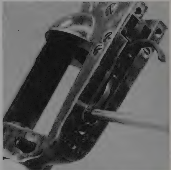
The Colt single-action has a trigger-locking bolt spring with two leaves. Remove the screw and inspect the spring.
