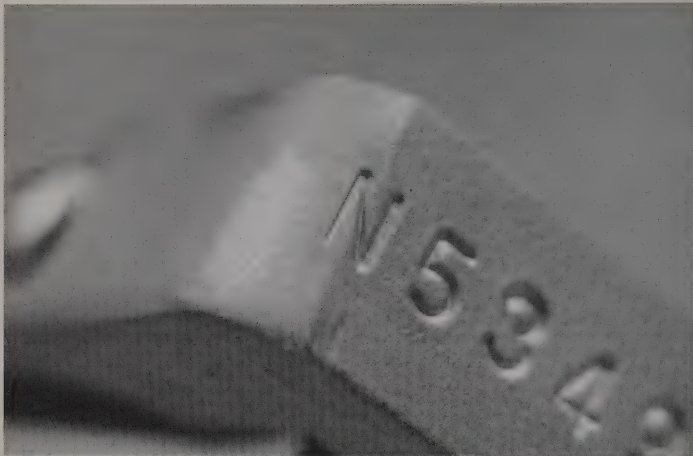
The frame was rounded, and the serial number survived. Measure yours before you go cutting, or you may have a slight problem.
