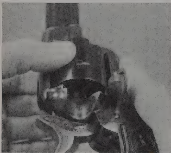
Thumb the hammer back to the second notch, open the loading gate and rotate the cylinder.
