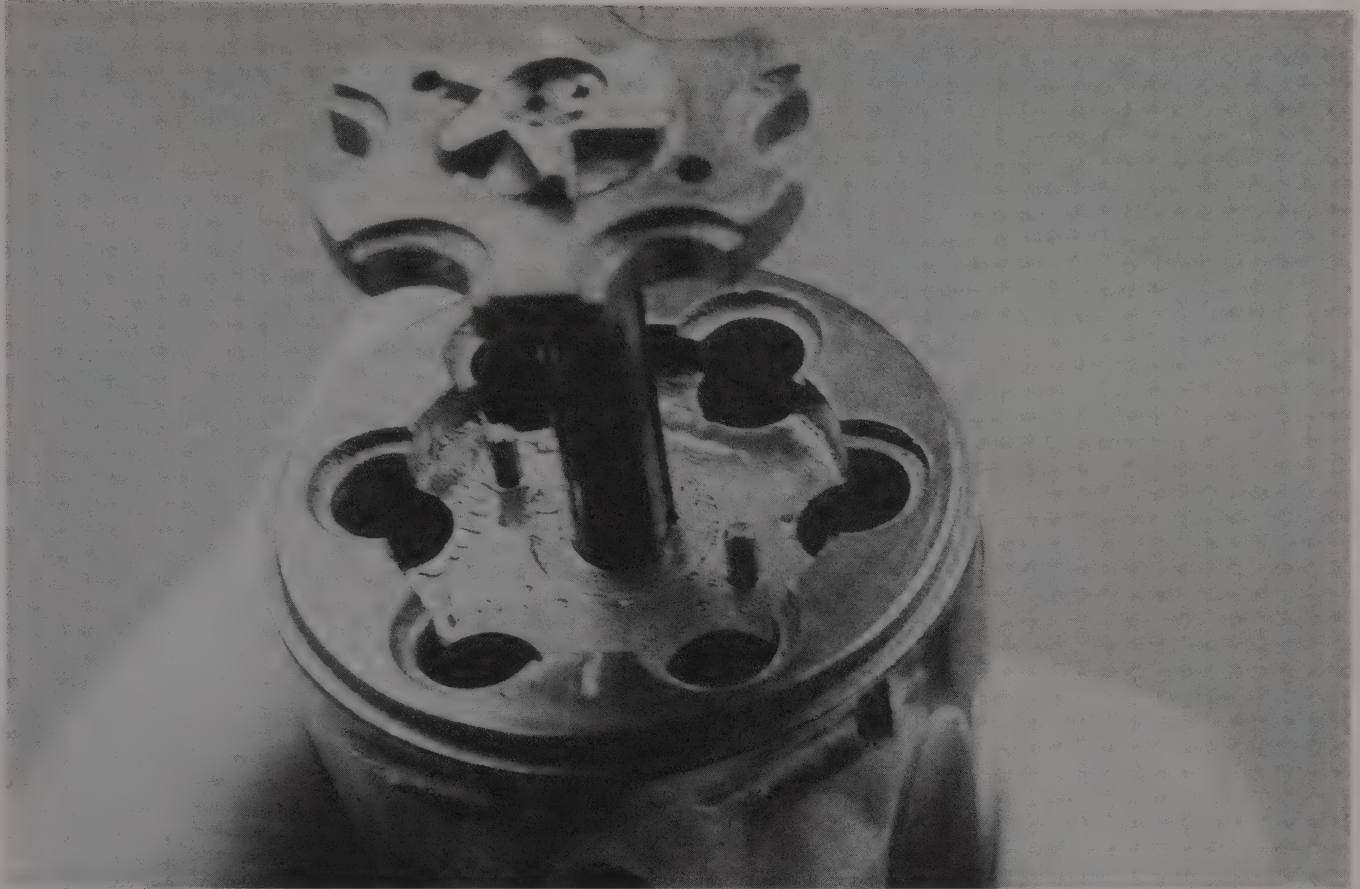
Powder residue or unburned flakes of powder under the extractor star will keep the cylinder from closing. Brush them out to close the cylinder.
