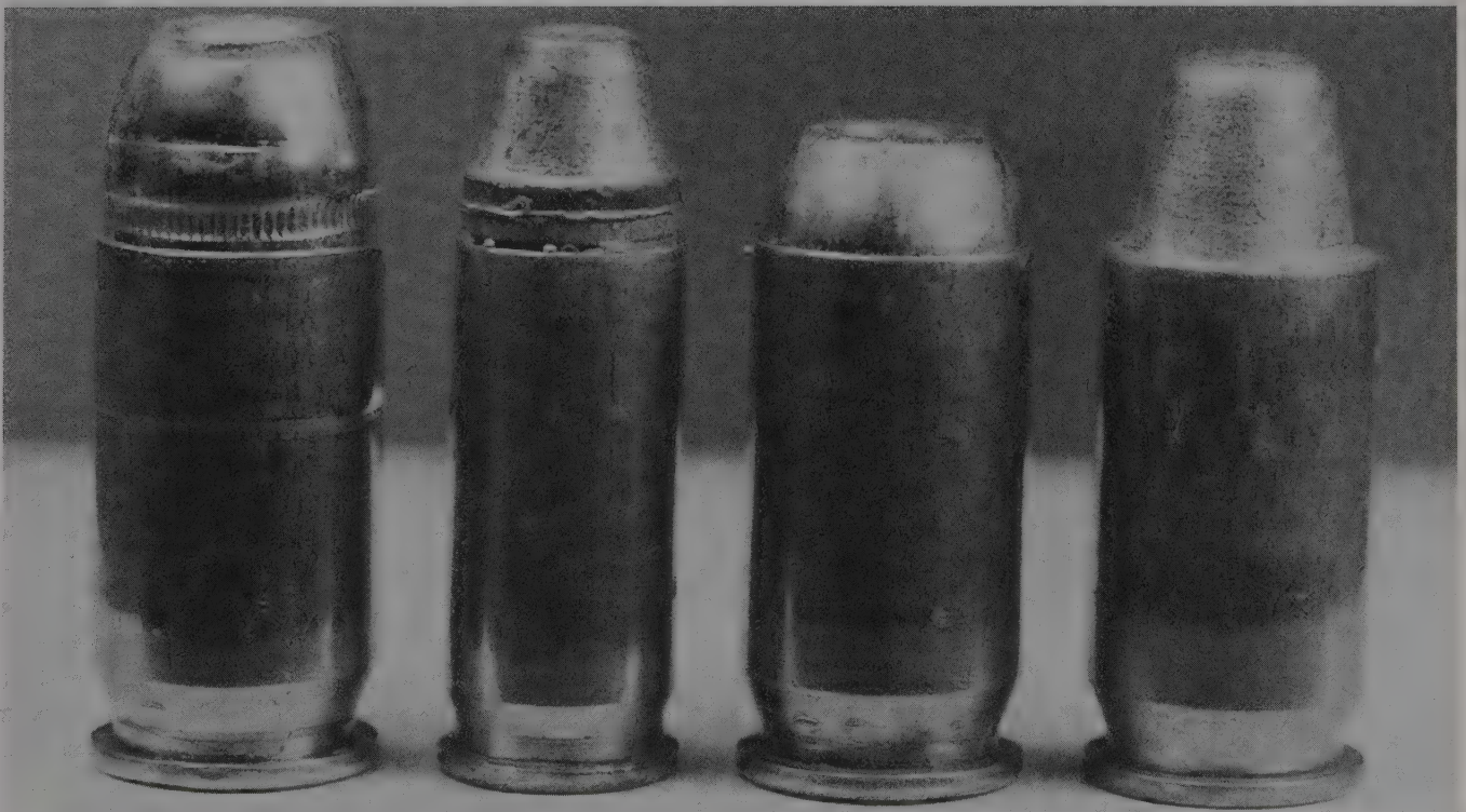
The two rounds on the right have bullets seated too deeply. The two on the left have bullets that are not deep enough. None will feed worth a hoot. If your reloads look like this, do not blame your pistol for not working reliably.
