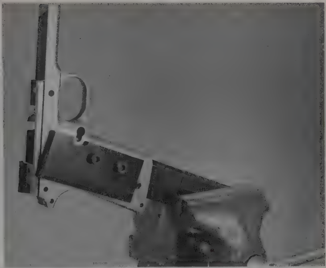
On the Wilson frame holder, the sideplate clamps the frame to the bar. You can work in the top, front, back and left side without interference.
