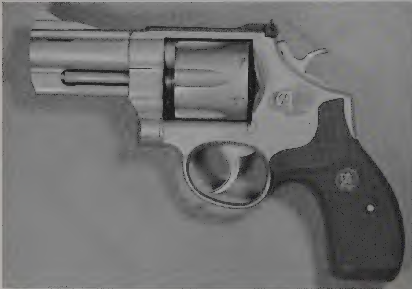
This revolver started life as a 6-inch .357 square butt N frame. It is now a round butt, .45 ACP snubbie. And it is plated with Armoloy and ported by Mag-na-Port. A complete transformation for a police trade-in.
