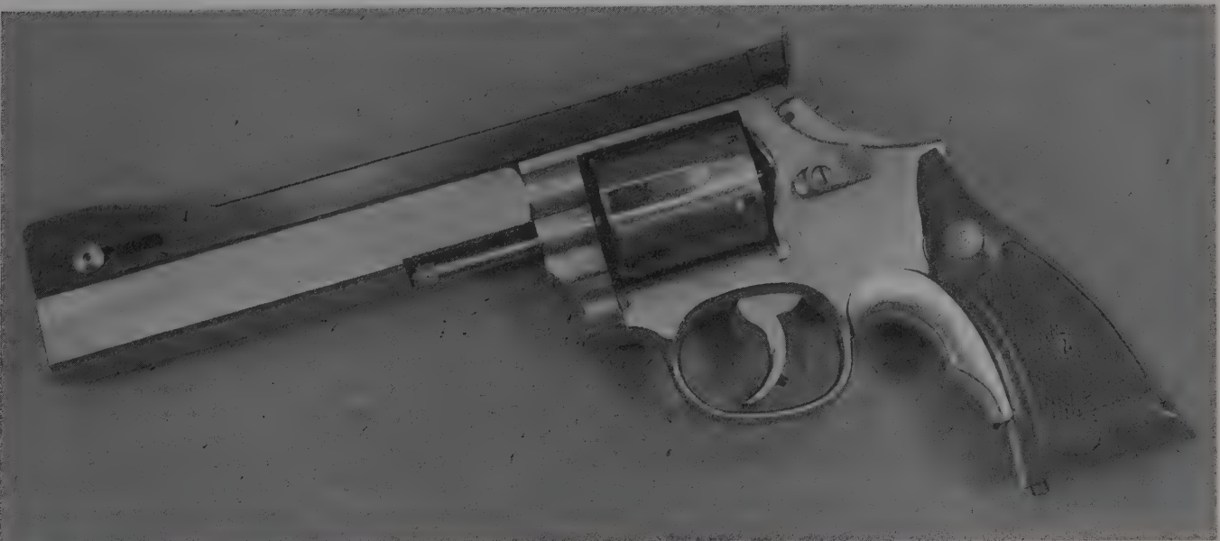
This Smith & Wesson is a tack-driver, with a slicked-up trigger pull, Barnett barrel and Aristocrat rib.
