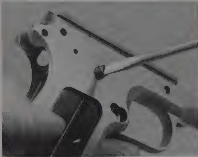
You have to remove the top grip screw bushing to clamp on the side plate.
