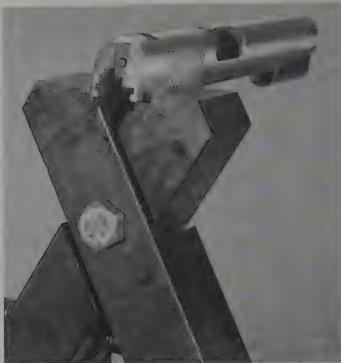
The slide has to be squeezed at the rear as well as the front part of the frame rails.
