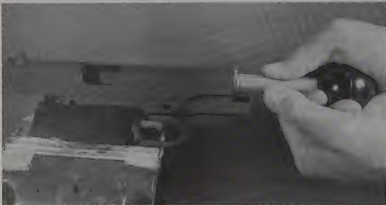
After putting lapping compound on the rails, move the slide back and forth to ease the tight spots and polish the surfaces.
