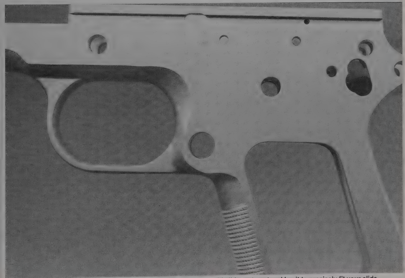
You can get frames with over-sized rails, to take up the slack of an old slide, or to cut and lap it to precisely fit your slide.
