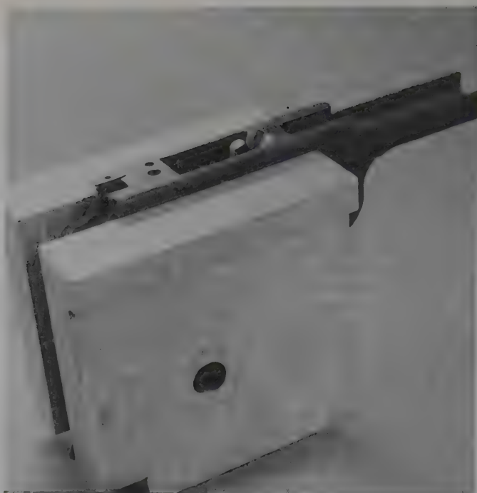
To swage, you must have frame holders like this Weigand set. You cannot swage while holding the frame in one hand, as you can peening.
