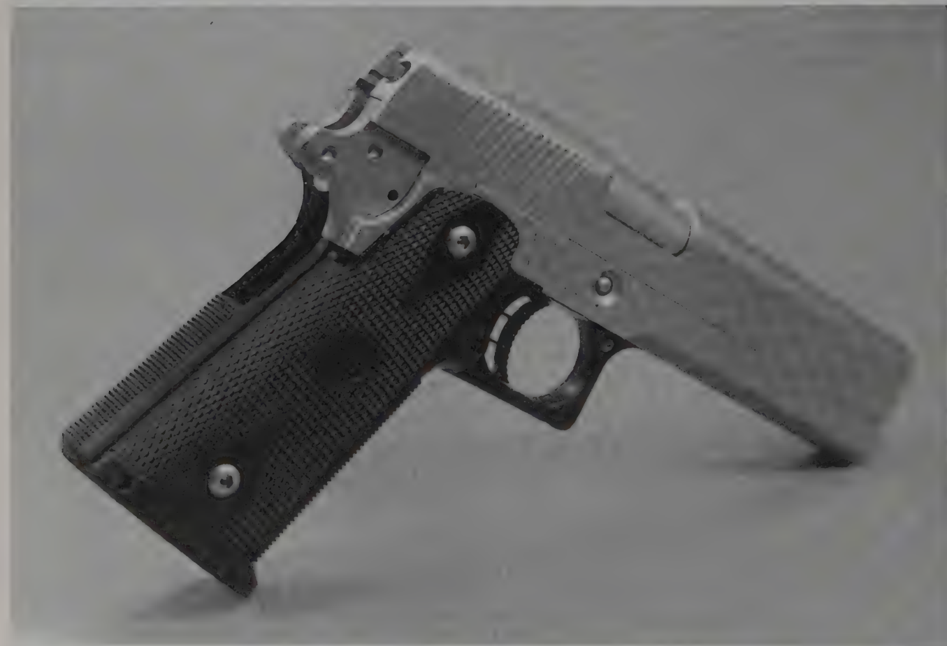
The STI Short Block has all the hard work done. The slide, frame and barrel have all been fitted. You need to put sights and internals in it. A great deal, and a great pistol.
