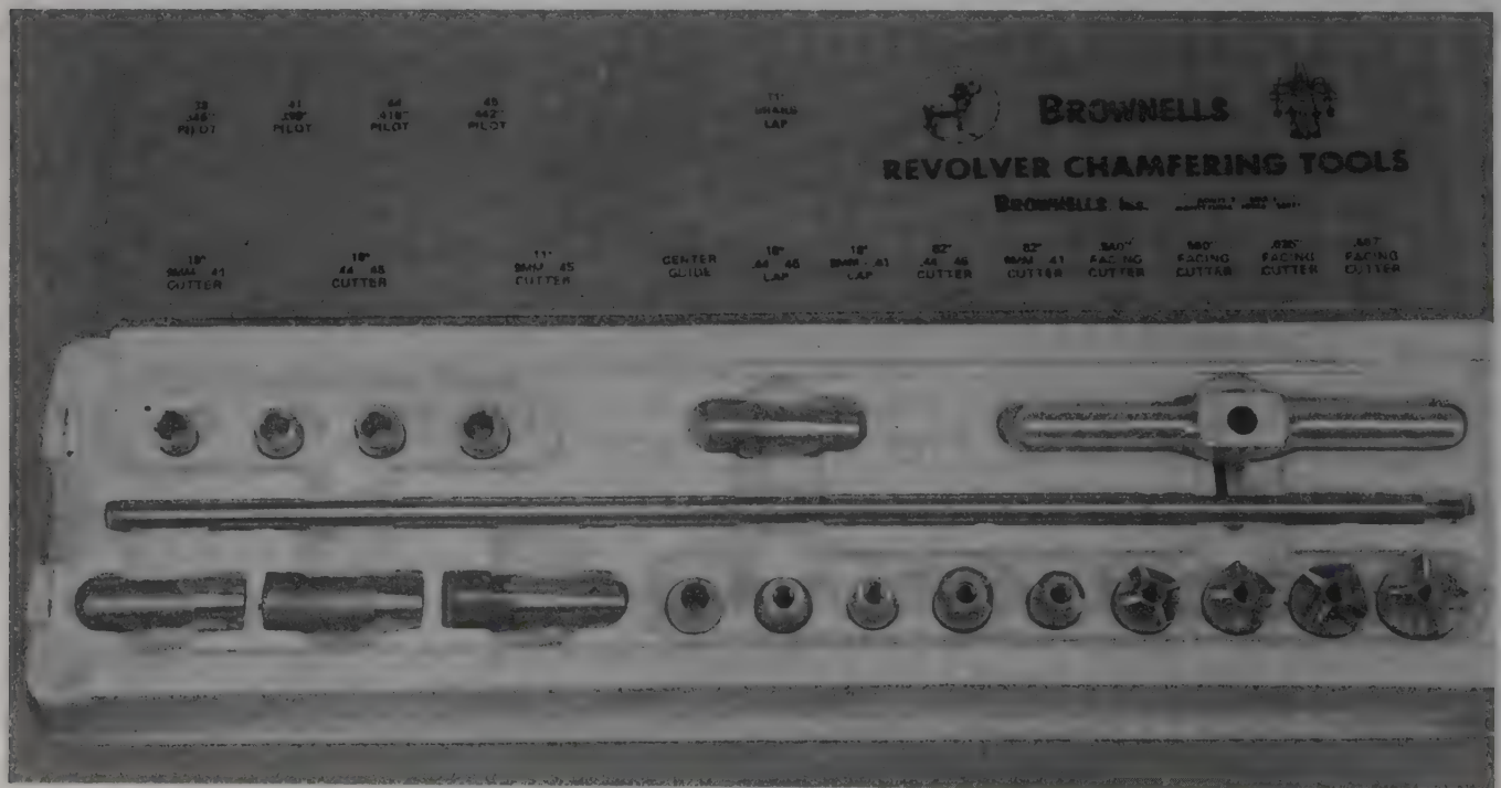
Brownells makes a kit that squares the barrel face and cuts the forcing cone. It works on barrels from 9mm to .45.
