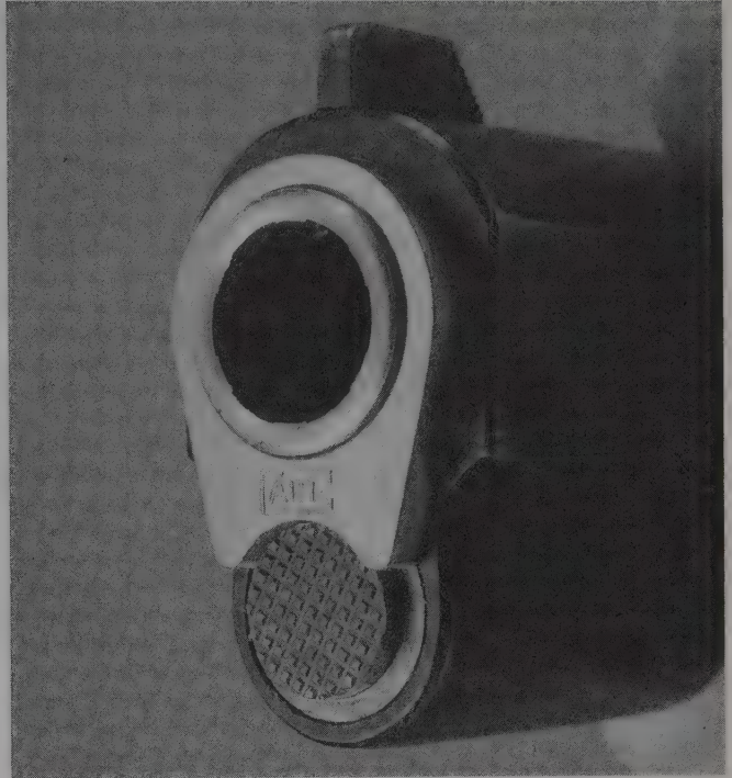
Here is the Kart match bushing included in the kit. With a properly fitted bushing up front and a tight fit in the rear, you will get the full benefit of a match barrel's accuracy.
