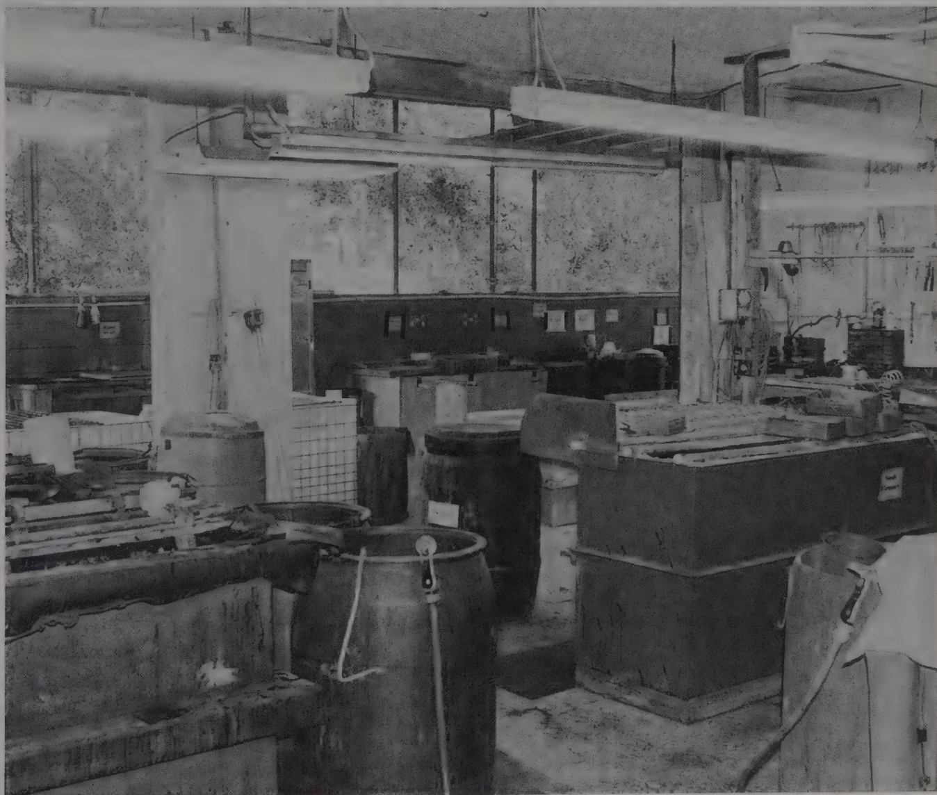
Large tanks of chemicals require good ventilation. Those aren't windows in the background, that's open air.
