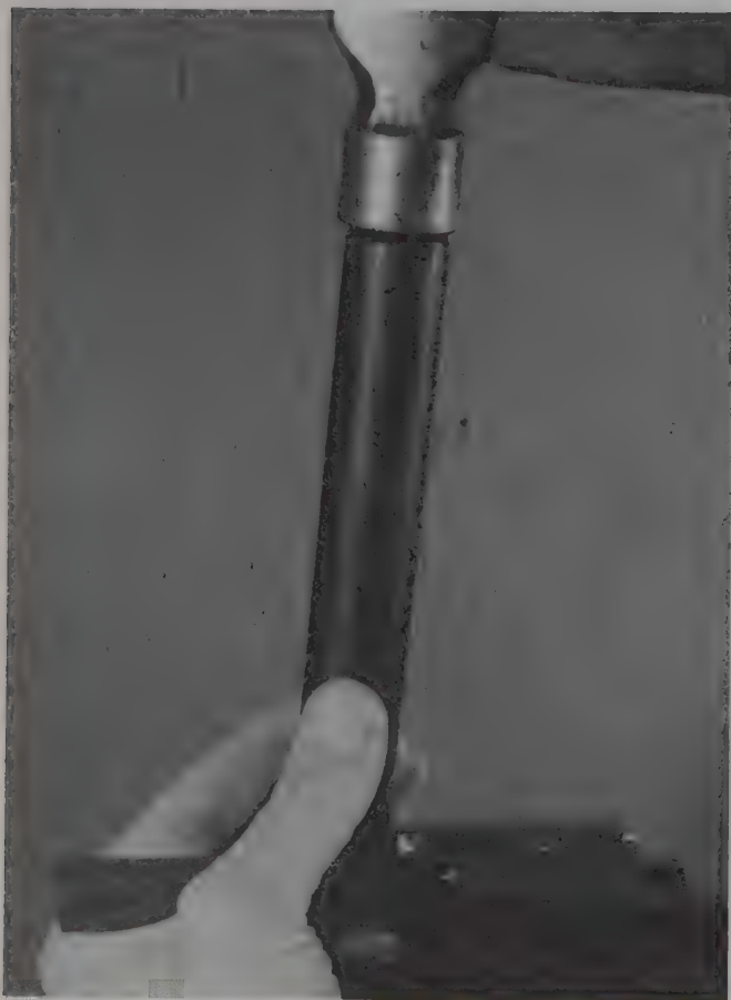
Strike the swaging bar to move the frame rails down to the forming bars.
