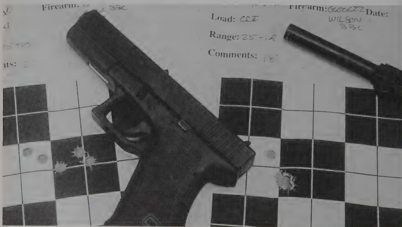
The standard Glock barrel is accurate. The Wilson barrel is even more accurate, and handles lead bullets too. The flier on the right-hand target is probably the shooter's fault.
