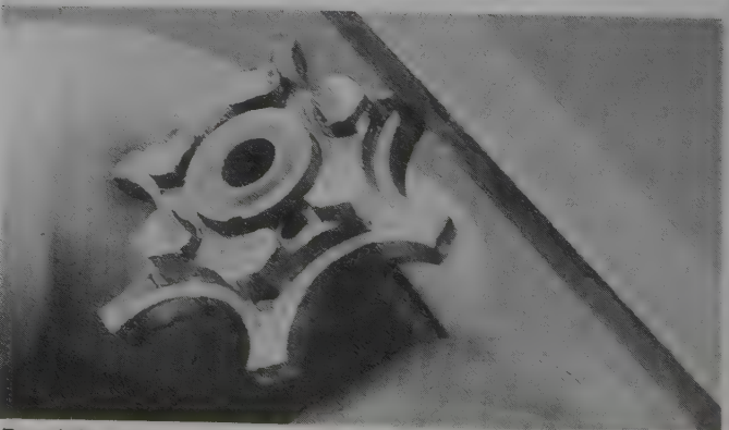
Bevel the corners of the extractor star with your pillar file.
