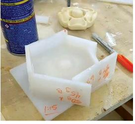
job, but the box can be easily snapped apart after you extract the mold. Andy also writes the weights for his part A and part B mold mixes right on the box, along with what time he can de-mold (1:15
