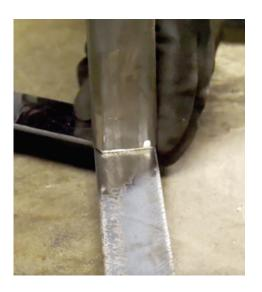
ensure a solid, sturdier weld. He also points out that you should spotweld around your entire workpiece first and then go back and completely bead the weld. This can help prevent warping of the metal as the surfaces are unevenly heated. **[BC]**
