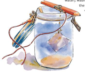
In about 45 minutes, you'll have a nickel-plated piece. Copper and zinc plating work the same way. For copper, first nickel-plate your part in nickel electrolyte and then plate in a copper electrolyte bath that you have prepared in exactly the same way as you did the nickel bath. Once you've created these electrolytes, you can keep them and use them over and over again as long as they're in an airtight container. See Geoffrey's video for more information: youtu.be/G-PtnwtOR24. **[GC]**
