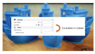
wide the lines of extruded material are," he says. "Higher values require more pressure to squeeze the molten filament out of the nozzle that also presses the layers together. I investigated how different extrusion widths impact quality and strength of our 3D prints and discovered that this might be a way to produce strong prints in a short amount of time." [SH2]
