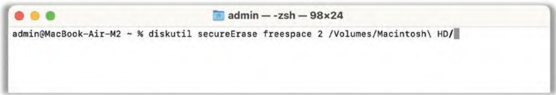
Figure 6-65. macOS Ventura Terminal secureErase freespace command
