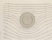
Figure 54: Streamlines for potential flow with circulation past a rotating cylinder. The cylinder experiences a downward Magnus force (see text).
