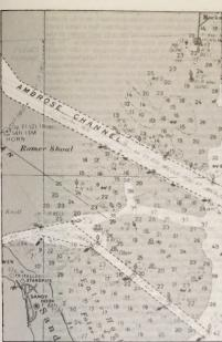
Figure 4: Small section of a large hydrographic chart (U.S. Coast and Geodetic Survey No. 1215) of the approaches to New York harbour. The scale is 1:80,000.
