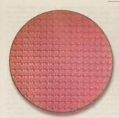
Figure 29: Using a 0.13-micron process, Intel can produce some 470 Pentium 4 chips from each 300-millimetre silicon wafer. right Intel Corp
