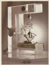
Figure 1: The first transistor, invented by American physicists John Bardeen, Walter Brattain, and William Shockley. Lucent Technologies Inc /Boll 1 abs
