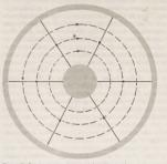
Figure 7: Cross section of a coaxial cable carrying high-frequency current.
