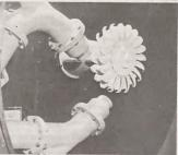
Figure 4: Pelton water turbine with twin jets.
