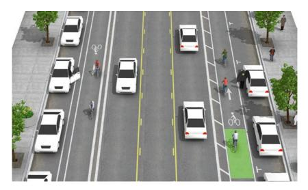
**Fig. 8.4** NACTO translates roadway design criteria—from AASHTO or the MUTCD—in a more accessible format for non-engineers, including design of buffered bike lanes. From *Urban Bikeway Design Guide* by National Association of City Transportation Officials. Copyright © 2014 NACTO. Reproduced by permission of Island Press, Washington, DC
