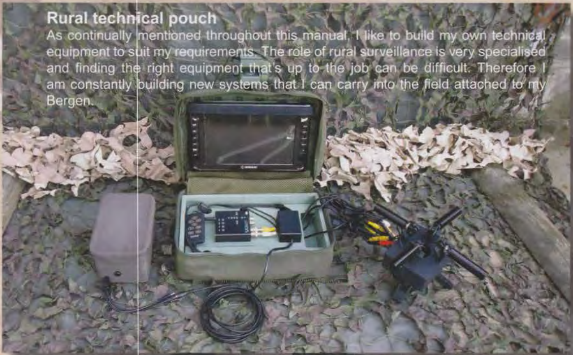
Covert camera with IR floodlight supported on a mini tripod
