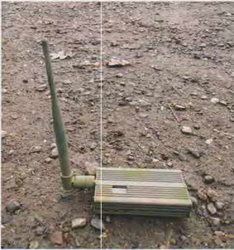
Above, low powered 2.4 GHz transmitter, this operates at 200mWatts. The range of this would be no more than 80 metres, line of sight.
