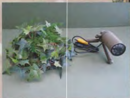
This covert bullet camera was deployed to trigger movement in a driveway. Shot from 2m.
