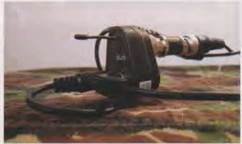
Above, low powered 2.4 GHz transmitter, this operates at 200mWatts. The range of this would be no more than 80 metres, line of sight.
