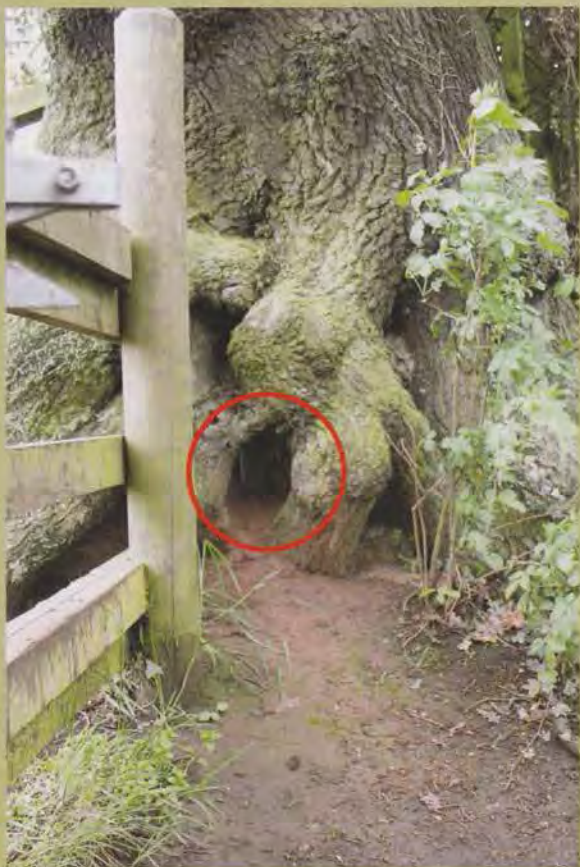
The sensor was concealed behind natural foliage with only the PIR window visible
