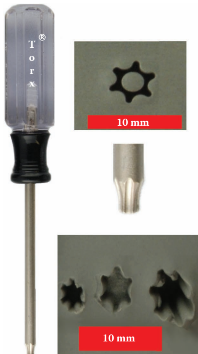
Figure 9.5 Torx is a type of screw head characterized by a six-point, star-shaped pattern. A variant of the Torx screw head is the Torx plus, an impression of which can be seen at the top right of this figure. Torx screws are commonly found on automobiles, computer systems, and consumer electronics, and are also becoming increasingly popular in construction. Close-up impressions of the Torx tip made in No. 2 Roma Plastilina sculpting clay are shown along with an enlargement of the Torx tip.
