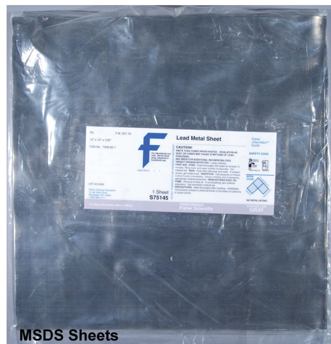
Figure 6.8 Pliable lead sheets 12 × 12 in. square, and 1/32 in. thick are available commercially and should be supplied with a materials safety data sheet (MSDS).
