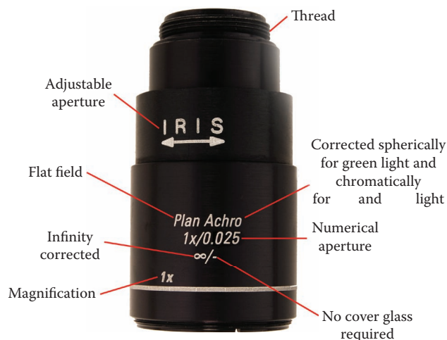
Figure 2.19 Above is shown a Leica® plan achromatic, fixed magnification, fixed NA objective lens.
