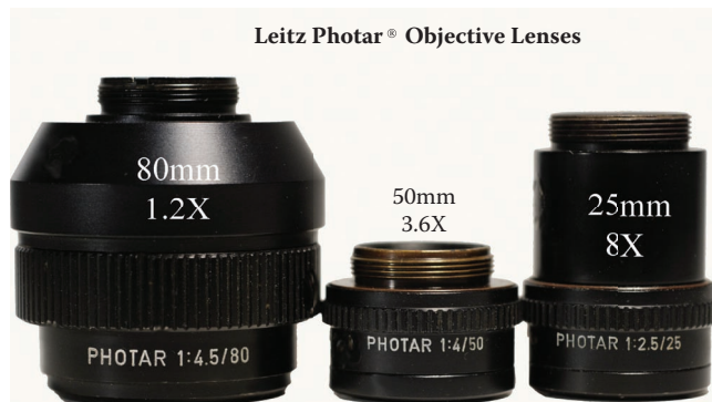
Figure 2.15 Three Leitz Photar® macro lenses provided with RMS screw thread for use in photomicrography and with comparison microscopy. The range of magnification of these three lenses is ideal for use in toolmark comparisons.
