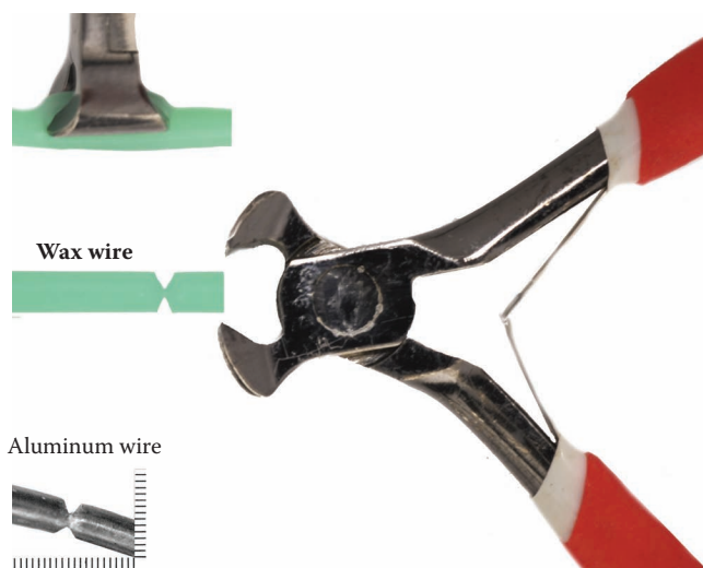
Figure 9.91 End-cut wire cutters cut both ends of wire into wedge shapes.
