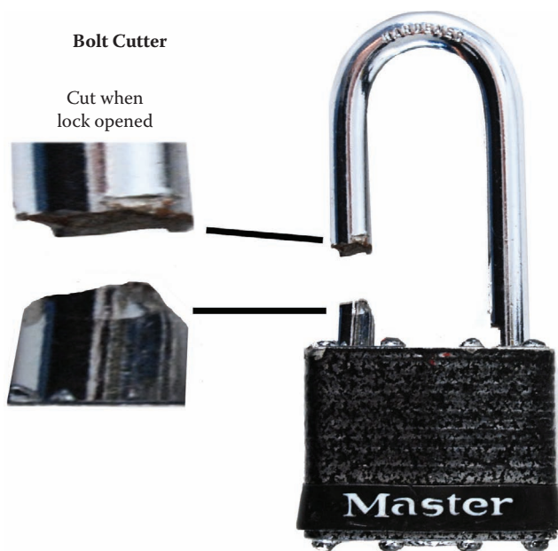
Figure 9.96 A staged burglary in which the lock's shackle was cut while opened with a shearing action bolt cutter.
