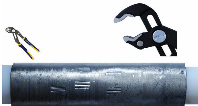
Figure 6.12 Standard test impressions of the teeth of Irwin™ groove-lock pliers made on a lead sheet wrapped around a section of PVC pipe.
