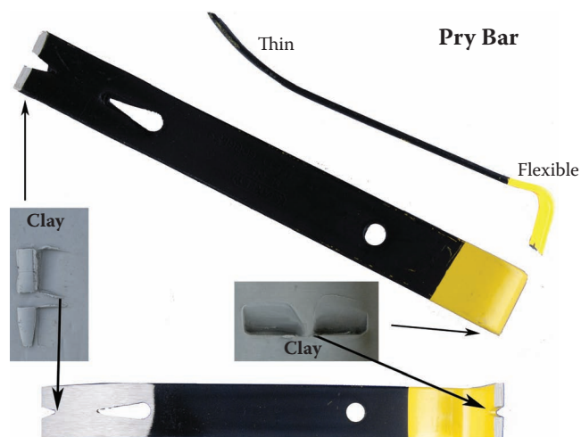
Figure 9.22 A pry bar and its common toolmarks in clay.
