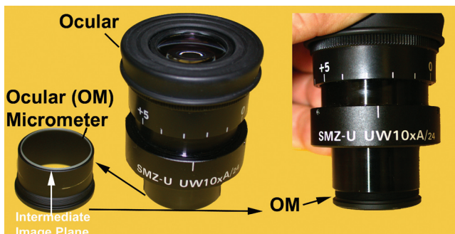
Figure 4.4 The placement of an ocular scale at the intermediate image plane of the eyepiece.
