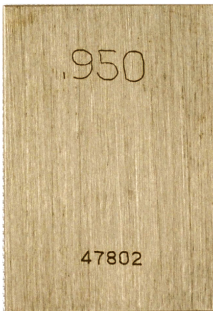
Figure 3.5 A NIST-traceable gauge block standard with its serial number and certified dimension marked on its front surface.
