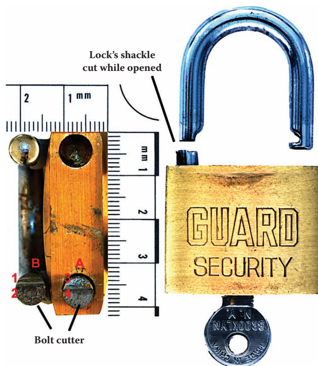
Figure 7.22 Based upon the physical appearance of the ends of the shackle marked B 1 and 2, and A 3 and 4 (on the left), it is evident that a bolt cutter was employed to cut the shackle from the lock. The position of the portion of the padlock's shackle (A) still within the lock casing is indicative of the shackle being cut while the padlock was in the open position.
