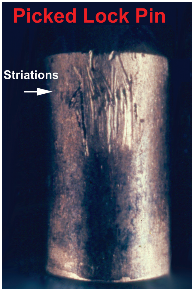
Figure 2 Pick marks on a tumbler pin removed from a lock cylinder. These marks suggest professional lock picks were used and not some makeshift device such as a paper clip.
