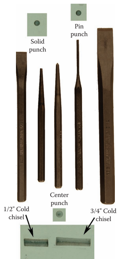
Figure 9.118 An assortment of common punches and chisels with their marks.
