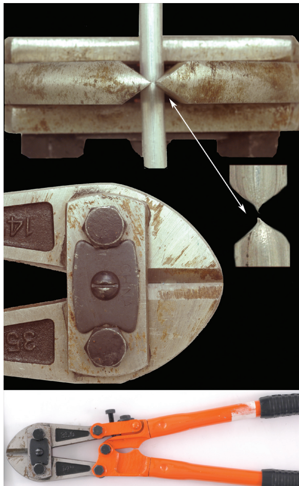
Figure 9.95 The cutting action of a center cutting blades (point-to-point) bolt cutter is depicted.
