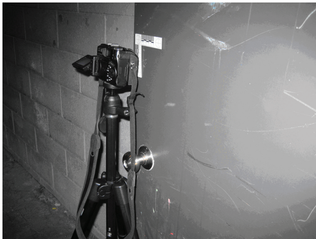
Figure 5.4 When taking close-up photographs, the camera should be mounted on a tripod, level, and held parallel to the plane of the surface bearing the toolmarks. Photographs should be taken with and without a scale.
