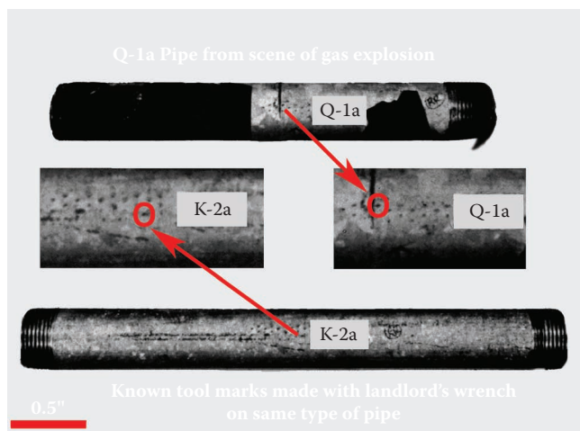
Figure 7.7 Two gas pipes, one (Q1a) from the scene of a homicide and gas explosion investigation, and one with known toolmarks from the landlord's basement (pipe marked K2a).
