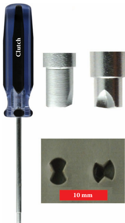
Figure 9.7 Clutch-head tips have four points of contact. They lock into the screw head when turned counterclockwise. The driver is unlocked by turning it in the opposite direction. Because of the many contact points, the tip will normally not damage the screw's head. Close-up impressions of the clutch tip made in No. 2 Roma Plastilina sculpting clay are shown along with an enlargement of the clutch tip.
