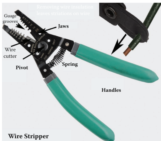
Figure 9.140 Common wire stripper used to cut various gauges of wire, as well as, crimp, and remove the insulation from electrical wires.
