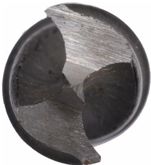
Figure 9.129 Countersink bits cut holes into material in order that screws and bolts can sit flush with or below the surface of a finished piece.
