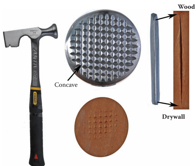
Figure 9.57 A drywall hammer.
