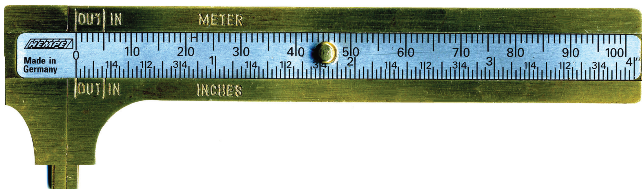
Figure 3.13 A common slide caliper, which allows for the acquisition of direct inside and outside linear measurements.
