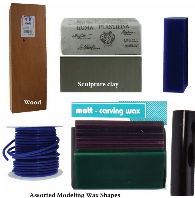
Figure 6.11 An assortment of materials needed for the replication of toolmarks, including modeling waxes, wood, and sculpting clay.
