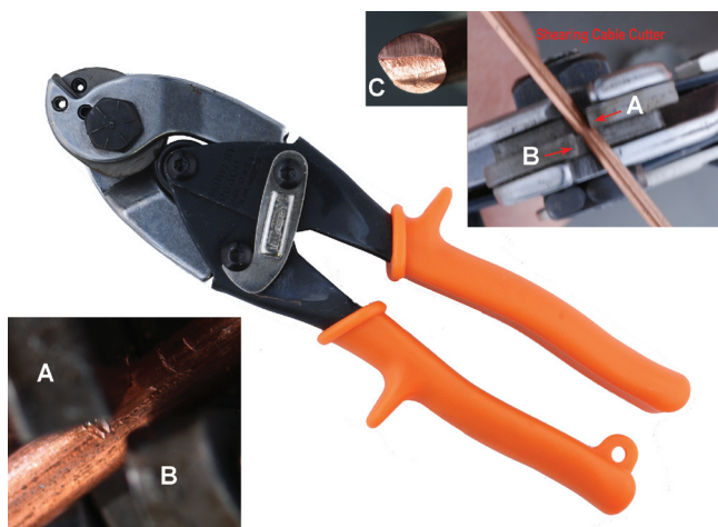
Figure 9.97 The shearing cutting action of a cable cutter blade (A) pushes the metal in one direction while blade B pushes the metal in the opposite direction until the cable fatigues (C).
