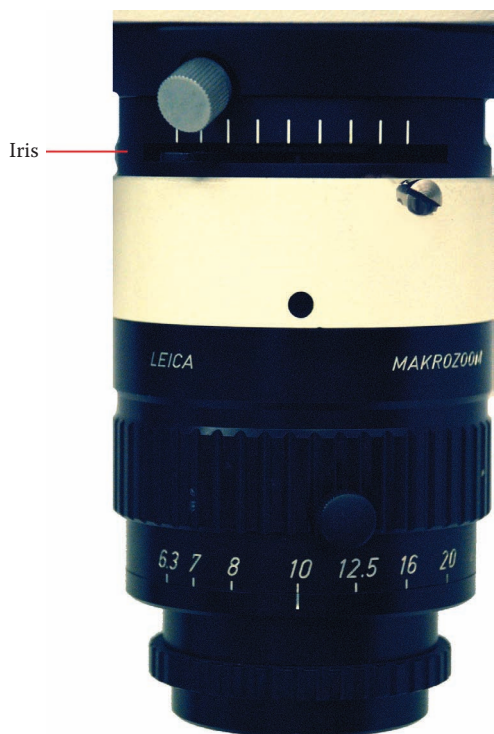
Figure 2.17 Shown is a Leica Makrozoom® achromatic objective lens used on many of Leica's modern comparison microscopes. This lens has a magnification range from 0.8 to 8.0×. The iris diaphragm is placed at the top portion of the lens and is used to control the intensity of the illumination and the depth of focus achieved in the final image.
