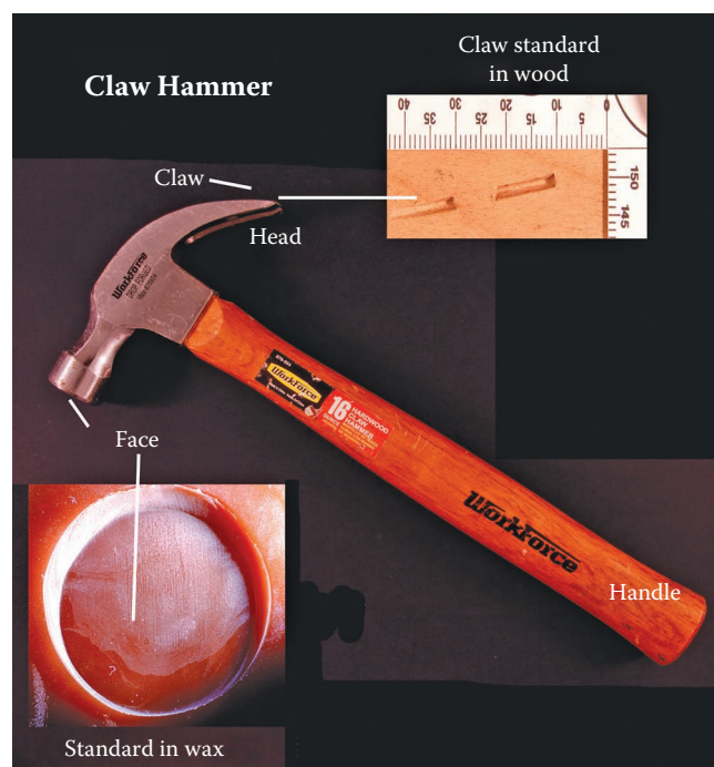
Figure 6.15 Red wax and wood test standards were made with a claw hammer in the same manner as the tested standards were prepared in Figure 6.14.
