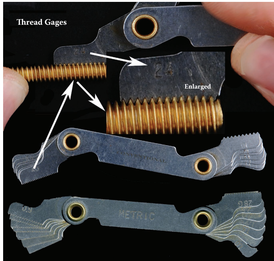
Figure 3.26 A screw is examined to determine its thread size.
