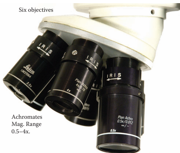
Figure 2.18 A set of Leica plan achromatic objective lenses. Each has a fixed NA, a fixed magnification and a built in iris diaphragm. The range of magnification with a 10× eyepiece is 5.0 to 40×. The author prefers the use of fixed magnification objective lenses over the zoom type lens.
