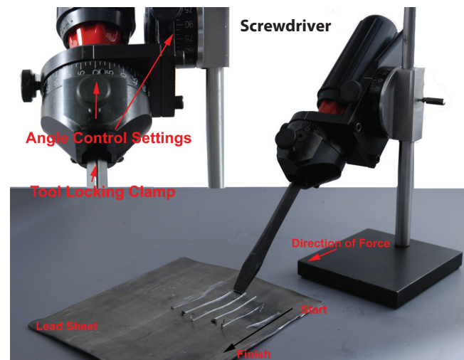
Figure 6.19 Preparation of screwdriver toolmark standards being made on a piece of lead sheet. An engraver's tool-sharpening holder with a variable height adjustment and two angle adjustments holds the test tool to make the exemplar toolmarks in the manner suggested by Burd and Kirk. 28
