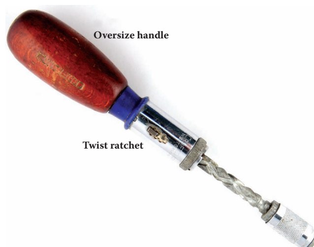
Figure 9.9 Mechanical screwdriver.
