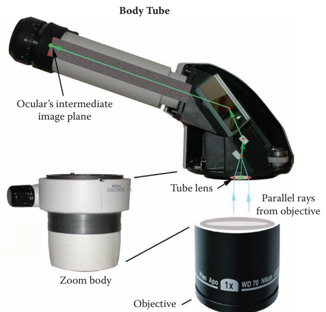
Figure 2.6 An archetypal body tube used in modern stereomicroscopes is depicted; note the presence of a tube lens at the base of the unit. Parallel rays exiting the objective or an intermediate optical device (zoom body) will be focused by the tube lens at the ocular's intermediate image plane.
