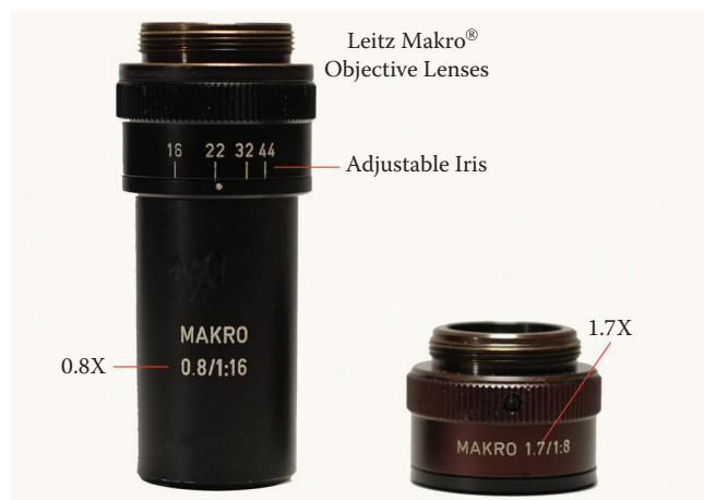
Figure 2.14 Two Leitz Makro® macro lenses provided with RMS screw thread for use in photomicrography and with comparison microscopy
