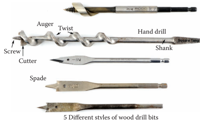
Figure 9.124 Five wood bits; the long auger bit is normally used with a brace, while the remaining four bits are used with electric drills.
