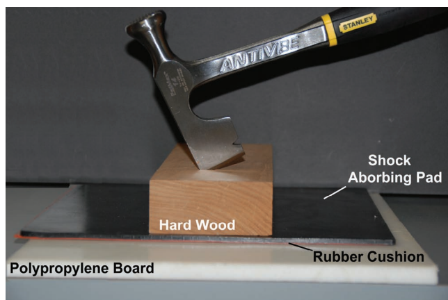
Figure 6.14 The preparation of test standards for hatchet, axe, drywall hammer, hammers, and other similar tools is usually accomplished as demonstrated above. A block of hardwood is placed on a piece of ½ in. polypropylene sheeting cushioned with a piece of shock-absorbing membrane and rubber pad, all positioned on top of a worktable. The wood is then struck with the subject tool.
