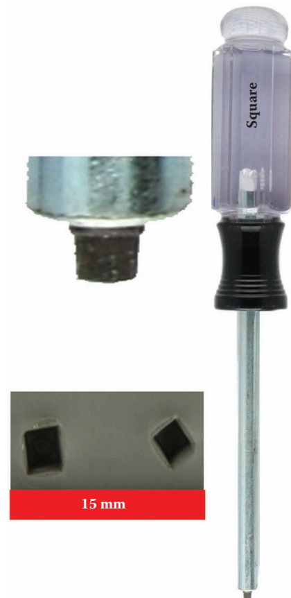
Figure 9.6 A Robertson screwdriver (also called a square drive screwdriver) is a type of screwdriver with a square-shaped tip. These screwdrivers are used mainly in Canada, but are growing in popularity around the world, because they are one of the most reliable screwdrivers. Close-up impressions of the square tip made in No. 2 Roma Plastilina sculpting clay are shown along with an enlargement of the Robertson tip.
