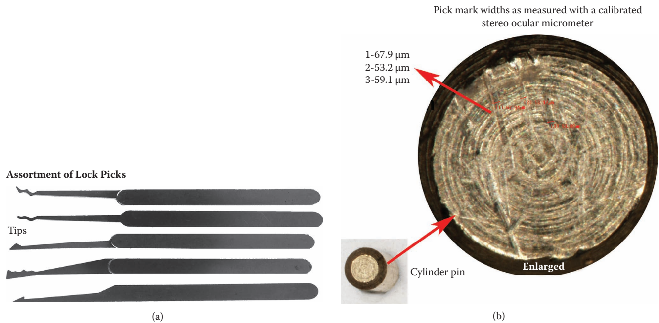
Figure 9.135 (a) Lock picks are made of thin, hardened steel, and they come in a large array of tip shapes. (b) A lock pin displaying pick marks indicating the lock cylinder it was removed from was picked.
