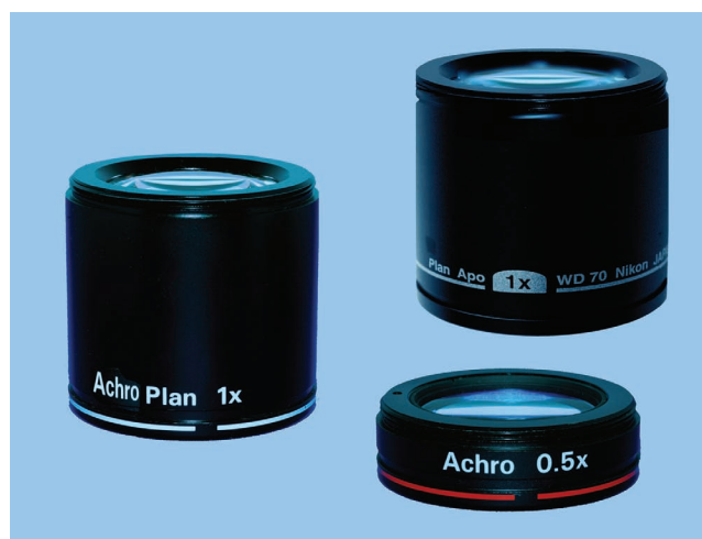
Figure 2.23 Shown above are two stereomicroscope plan achromatic common microscope objectives (corrected for flatness of field, 2 colors chromatically, and the color green spherically) and one stereomicroscope plan apochromatic common microscope objective (corrected for flatness of field, 4–5 colors chromatically, and 3–4 colors spherically).
