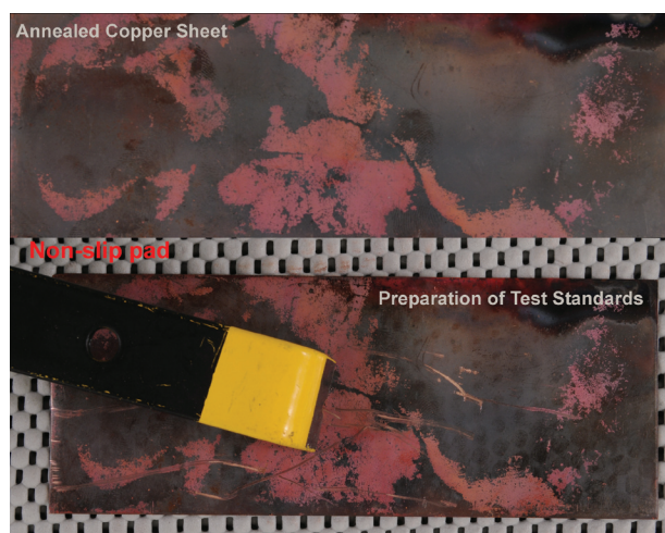
Figure 6.7 Top: An annealed copper sheet is placed on an antislip pad. Bottom: A pry bar is scraped along the metal's surface to produce known test toolmarks.
