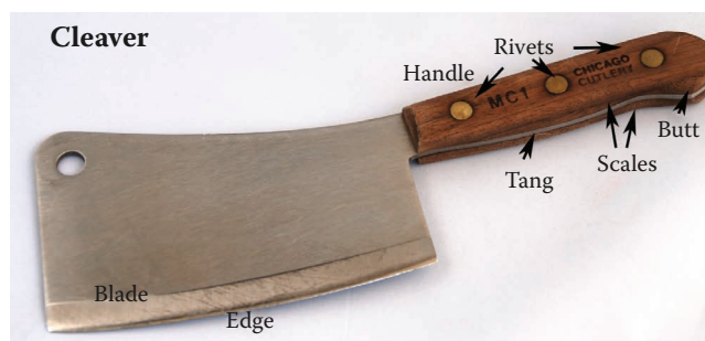
Figure 9.142 A cleaver, with its nomenclature, is often used in violent assaults. It makes toolmarks in skin and bone similar to those made by an axe.
