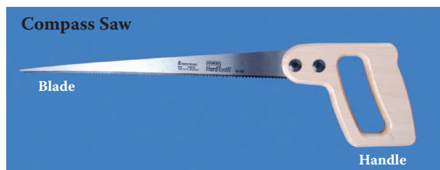
Figure 9.36 Compass or keyhole saw.
