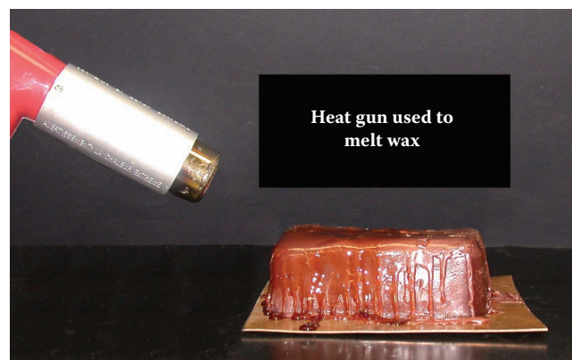
Figure 6.16 To remove heavy scratches or dents, gently heat wax surface with a heat gun and allow to air cool until it returns to its original consistency. Caution: Only melt wax in a fire proof well ventilated hood.
