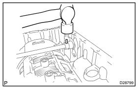
(c) Using a hammer, drive in a new spring pin.
