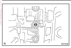
(b) Check that the oil pressure apply hole of the brake cylinder NO.2 aligns with the oil pressure apply hole of the transmission case.
