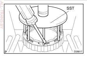
(c) Using SST and press, install the snap ring. **NOTICE:**
