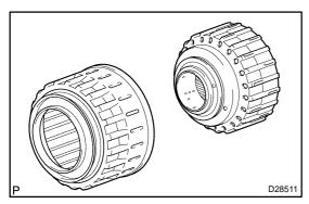
(c) Be careful not to damage the O-ring. Press in the clutch drum sub assy into the reverse clutch piston with both hands.
