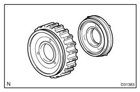
(b) Remove the coast clutch piston from the forward clutch piston.
