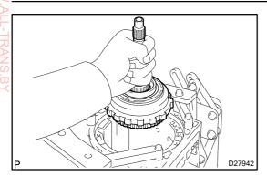
(b) Remove the intermediate shaft with the 1 way clutch assy No.3 from the case.
