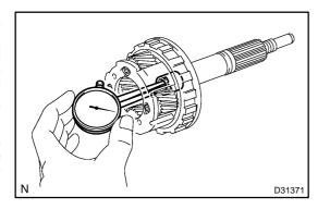
(b) Using a dial indicator, measure the inside diameter of the rear planetary gear bushing.
