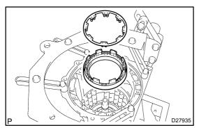
(a) Remove the brake piston return spring and the brake piston No.1 with the brake cylinder No.1 from the transmission case.
