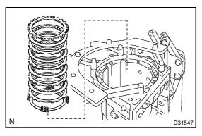
(b) Remove the 2 flanges, the brake piston return spring, the 4 discs and the 3 plates from the case.
