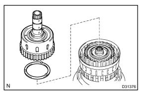
(b) Install the forward clutch hub sub assy to the clutch drum assy.
