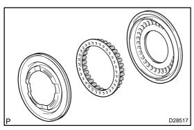
(c) Remove the clutch balancer No.2 and the direct clutch return spring sub assy from the direct clutch piston sub assy.
