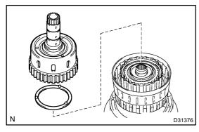
(b) Remove the 2 thrust needle roller bearings from the forward clutch hub sub assy.
