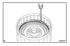
(b) Using a screwdriver, install the 2 hole snap rings on the clutch drum sub assy.
