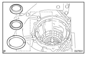
(b) Remove the thrust needle roller bearing, the thrust bearing race No.3 and the planetary carrier thrust washer No.2 from the front planetary gear assy.
