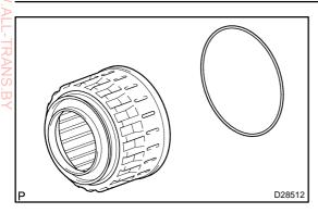
(b) Coat a new O-ring with ATF, and install it on the reverse clutch piston sub assy.
