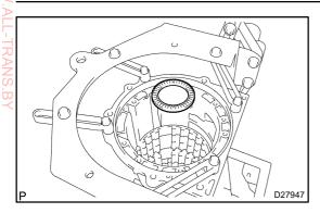
(c) Remove the thrust needle roller bearing from the case.
