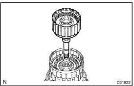
(b) Remove the input shaft assy from the clutch drum assy.
