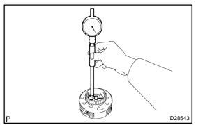
(b) Using a dial indicator, measure the inside diameter of the front planetary gear bushing.
