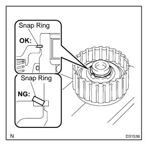
(e) Set the end gap of the snap ring in the piston as shown in the illustration.
