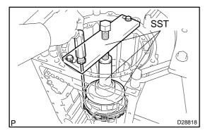
(b) Using SST and a press, install the brake No.2 spring snap ring.
