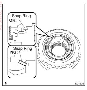
(c) Set the end gap of the snap ring in the piston as shown in the illustration.
