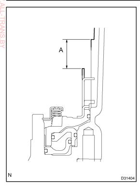
(b) Using vernier calipers, measure the level difference (length A) between the upper surface of the brake apply tube and the hitting surface of the brake flange No.4 at both ends across the 1st & reverse brake piston diameter, and calculate the average.
