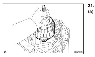
Remove the clutch drum & input shaft assy from the trans-(a) mission case.
