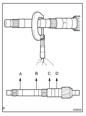
(b) Using a micrometer, check the outer diameter of the intermediate shaft positions shown in the diagram.
