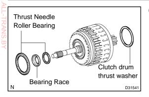
(b) Remove the clutch drum thrust washer, 2 thrust needle roller bearings and bearing race.
