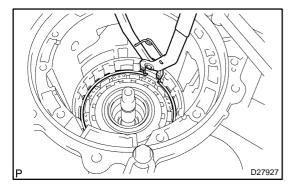
102. INSTALL 2ND BRAKE PISTON HOLE SNAP RING
