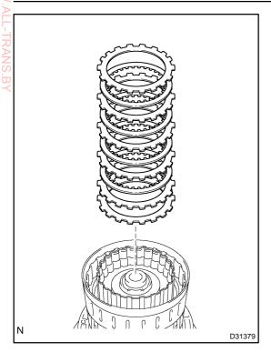
(b) Remove the flange, cushion plate, 4 discs and 4 plates from the input shaft assy.
