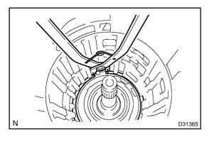
(b) Using SST, install the snap ring. SST 09350-30020 (09350-07050, 09350-07060)
