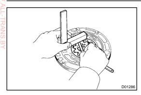
(d) Using a steel straight edge and a feeler gauge, measure the side clearance of both gears.
