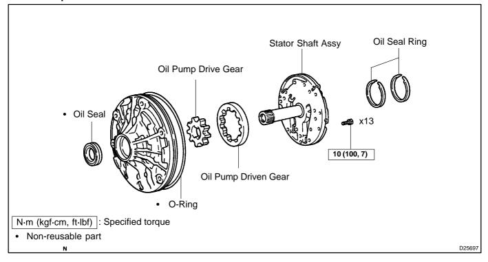
(d) Torque, oil applying position, and non-reusable parts are described as important points in the procedure.
