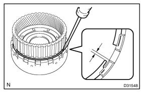
(b) Using a screwdriver, install the snap ring.
