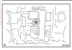
(d) Check that the oil pressure apply hole of the brake cylinder No.2 aligns with the oil pressure apply hole of the transmission case.
