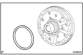
Remove the thrust bearing race No.1 from the oil pump. (c)
