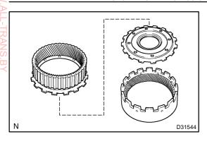
(b) Remove the CTR planetary ring gear and the front planetary ring gear flange from the front planetary ring gear.
