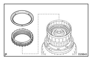
(b) Remove the reverse clutch reaction sleeve, the clutch cushion plate, the reverse clutch flange, the 5 reverse clutch discs, and the 4 clutch plates from the reverse clutch hub sub assy.
