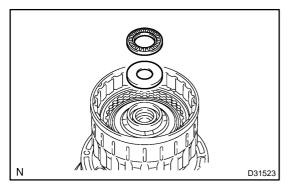
(c) Install the thrust needle roller bearing and thrust bearing race.
