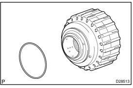
(c) Remove the O-ring from the clutch drum sub assy.
