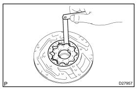
(c) Using a feeler gauge, measure the clearance between the driven gear teeth and the drive gear teeth.
