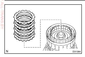
(b) Remove the flange, the 3 discs and the 3 plates from the input shaft assy.
