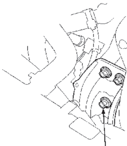
FRONT ENGINE MOUNT BRACKET BOLTS 38 N·m (3.9 kgf-m, 28 lbf-ft)
