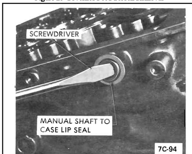
Figure 26 Manual Shaft Lip Seal Removal
