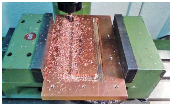
Figure 4 — The milled channel is for water cooling.
