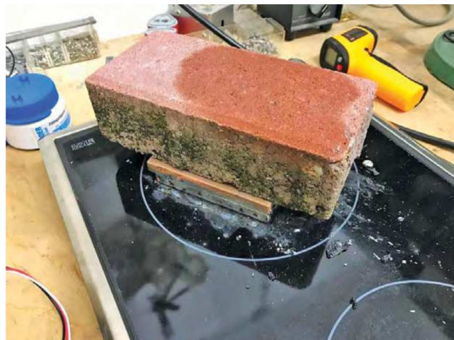
Figure 5 — The plates are soldered together.
