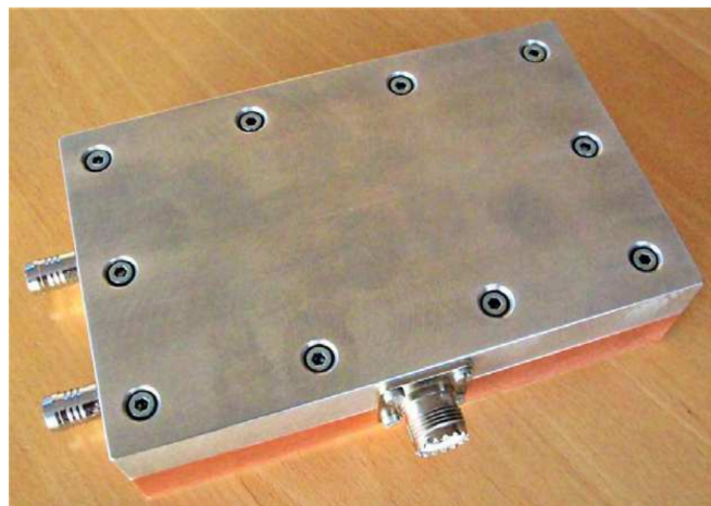
Figure 3 — The completed water-cooled dummy load, with the water intake/exhaust connectors on the left.
