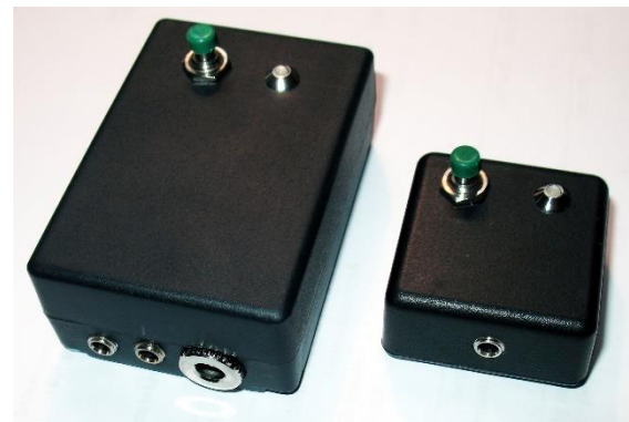
Figure 5 – Control unit with a single external switch module.
