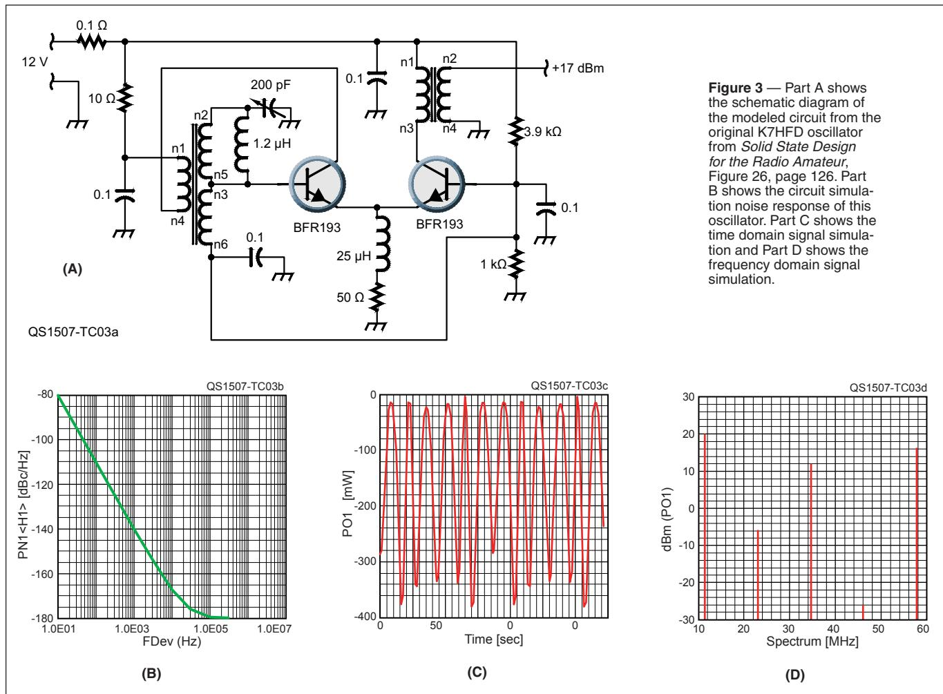
lator exhibits low phase noise. First is that the LC resonator is loaded by the transistors only when the resonator voltage swings through zero. The resonator thus operates very near its unloaded  $Q$  for the rest of the cycle. In the Leason model, using an amplifier matched to the resonator, the optimum loaded  $Q$  is  $\frac{1}{2}$  the unloaded  $Q$ . The upshot is that, at least in theory, the flank of the phase noise curve is thus pushed to the left by an octave.
