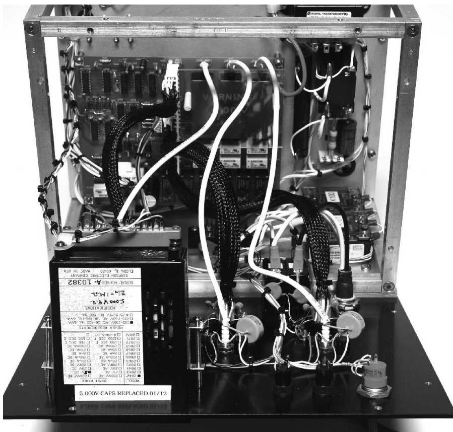
Figure 8 — The front side of the subpanel houses the controller printed circuit board, the low voltage transformer, and the step-start circuits.
