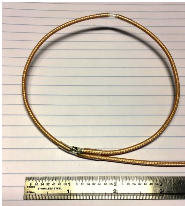
Figure 7. Completed pickup loop, about 3 inches diameter.
