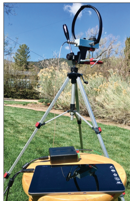
Figure 3 — A magnetic loop antenna (National RF HFDF Vector Gun) secured by a clamp to a tripod feeding an SDR receiver (SDRplay RSP2) connected to tablet PC (ASUS Transformer Mini T102) running SDRConsole .
