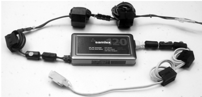
Figure 3 — A 12 V dc-to-120 V ac 1 A inverter with required RF filtering.
