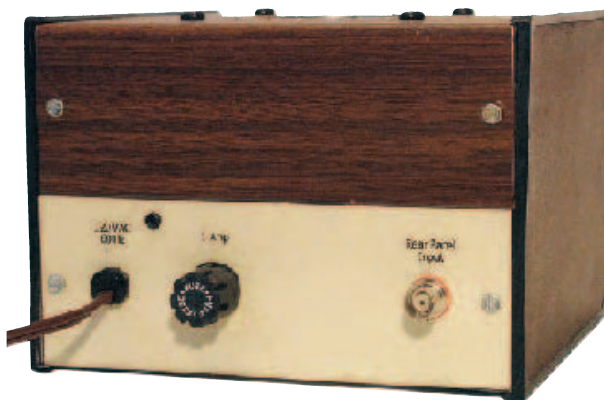
Figure 3 — Signal tracer rear panel. This legend was also prepared on clear film using Microsoft PowerPoint.
