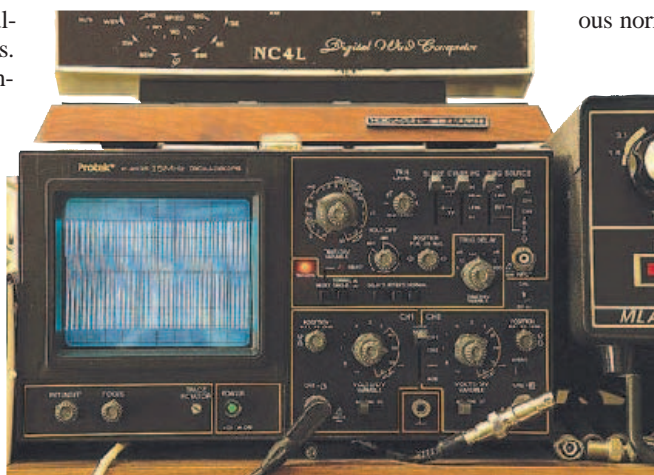
Figure 1 — An oscilloscope that is typical of those that can be purchased from eBay or at hamfests for $50 to $100. It is a dual channel 'scope with 35 MHz bandwidth — more than is usually needed.
