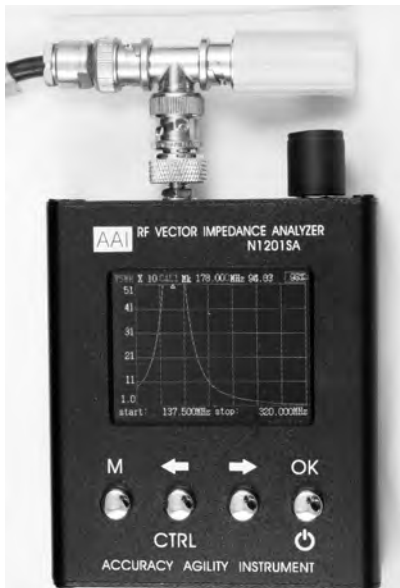
Figure 8 — Measuring resonant frequency of a stub
