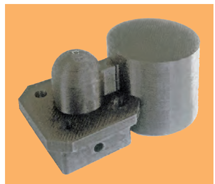
Figure 1 — Purpose-designed and 3D-printed plastic framework for an SO-239 VHF/UHF ground-plane antenna. The cylindrical cap at the right is sized to slip over the end of a \frac{3}{4} -inch PVC pipe mast. Four ground-plane radials bolt to the horizontal member at the left of the mast-mounting cap. The SO-239 coax connector bolts to the radial elements through the bottom of the radial mount with the antenna's vertical element soldered to the connector's center pin and projecting through the dome of the small cylinder atop the radial mounting plate. Silicone is injected through the small hole in the side of the radial mounting plate for waterproofing.
