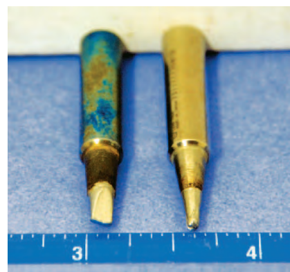
Figure 3 — The Mini Iron pencil tip (right) is preferred over a flat, wide soldering station tip (left). [Paul Cianciolo, W1VLF, photo]
