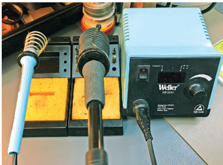
Figure 2 — The Weller model WM120 Mini Iron is on the left, and the model WES51 soldering station is on the right. [Dino Papas, KLØS, photo]
