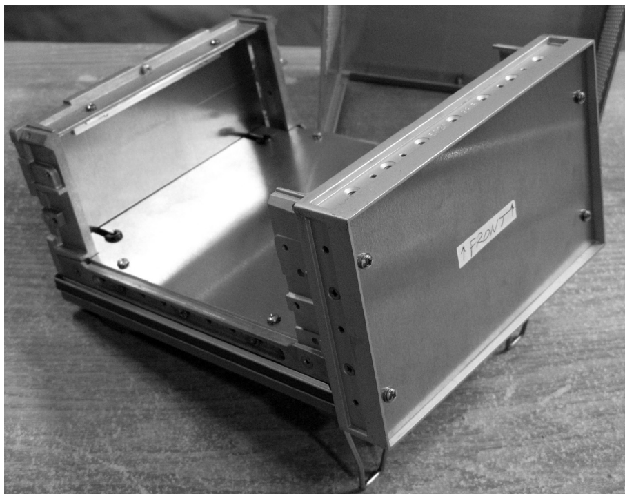
Figure 4 — Finished enclosure showing sheet aluminum panels installed.
