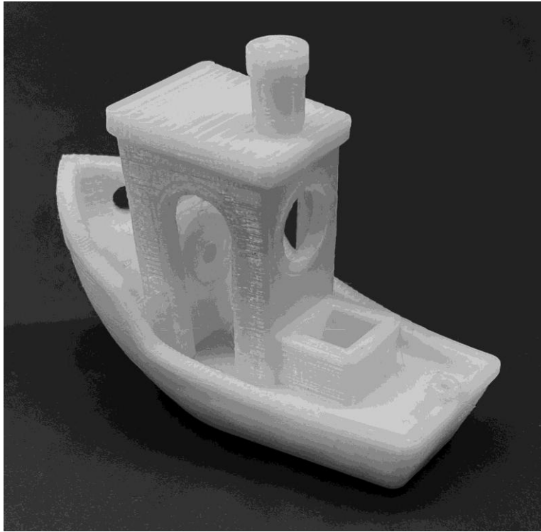
Figure 4 — Benchy, a popular advanced user’s test object to help fine tune printer settings via a slicer program
