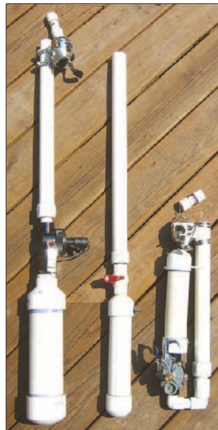
Figure 7 — Other types of valves and firing systems can be used. Right: Firing the sprinkler valve pneumatically. Center: a PVC globe valve.
