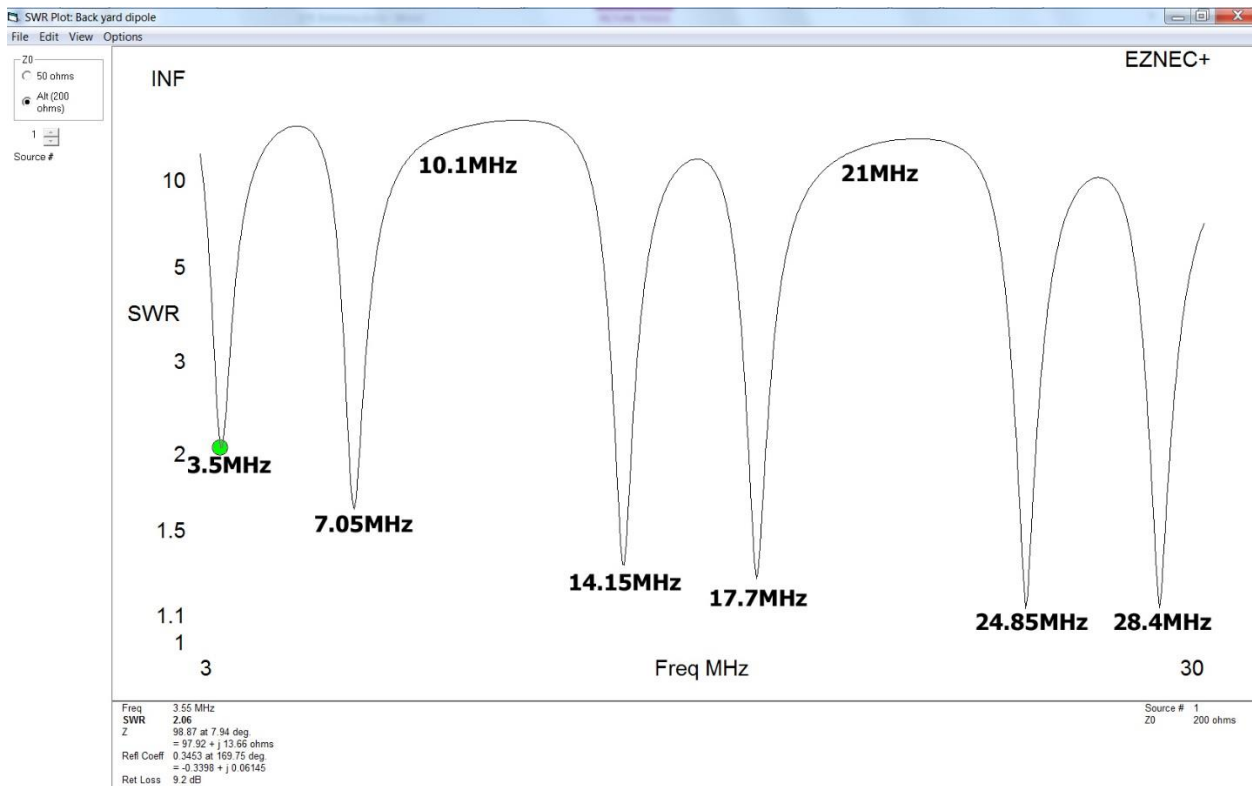
Figure 2 Simulated 200-ohm SWR plot of 1/3-fed 80m half-wave dipole
