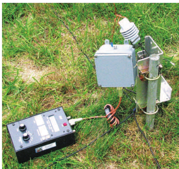
Figure 11 — An antenna analyzer is used in this typical test setup to adjust the matching of the antenna. The wire version is shown.
