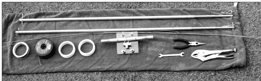
Figure 21.31 — The entire inverted-U antenna parts collection in semi-nested form, with its carrying bag. The tools stored with the antenna include a wrench to tighten the U-bolts for the mast-to-plate mount and a pair of pliers to help remove end wires from the tubing.
