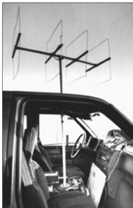
Fig 21.134 — KØOV uses this mobile setup for RDF on several bands, with separate antennas for each band that mate with a common lower mast section, pointer and 360° indicator. Antenna shown is a heavy gauge wire quad for 2 meters.
