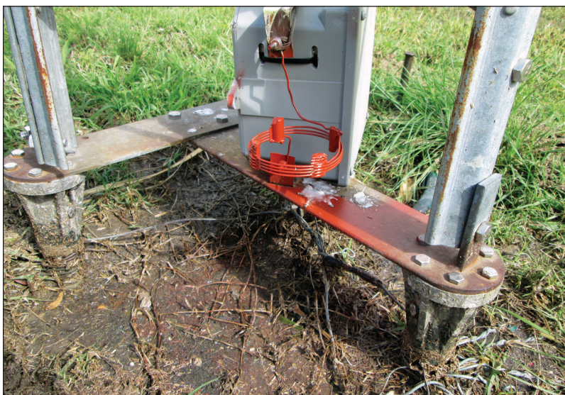
Figure 1 — Base-loading coil for switching between 80 and 75 meters is weatherized with Sprayon® EL601 Red Insulating Varnish Aerosol. The SWR did not change after applying the varnish.
