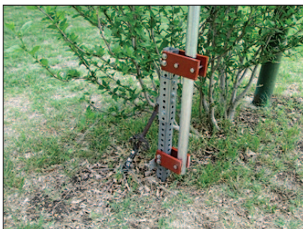
Figure 3 — Red high-voltage insulating varnish protects the fold-over insulators of a 60 meter vertical.
