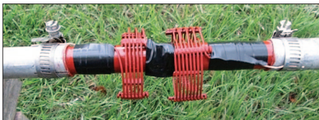
Figure 2 — Two series-connected coils surrounding a solid fiberglass insulator tube on a 60 meter vertical, after two coats of high-voltage insulating varnish.
