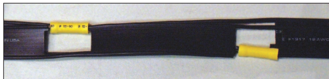
Figure 3 — A balanced line "long splice" with butt connectors, ready for crimping. By keeping much of the between-conductor web intact, it can be used to remove strain from the connections. For soft copper wire, a Western Union splice can be used, while copper-plated steel requires other measures, such as the crimp connectors shown.
