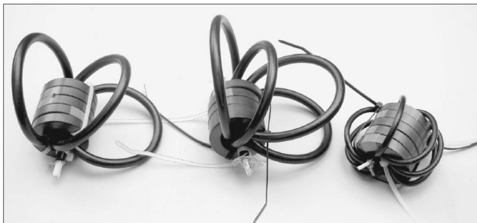
Figure 20.26 — Typical transmitting wound-coax common-mode chokes suitable for use on the HF ham bands.
