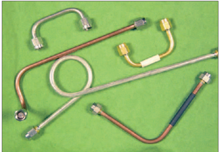
Figure 1 — Surplus semirigid cable assemblies come in all shapes and sizes.
