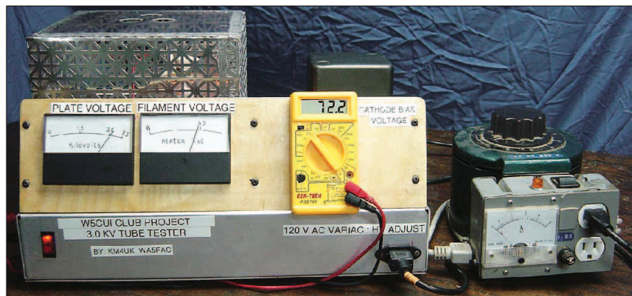
Figure 1 — The completed high power tube tester in use. The Variac to the right is used to incrementally increase the plate voltage and view the line current in the event there is a short or too high a current draw for a particular setting. The switch on the left below the meters separately turns on the filament voltage and fan.
