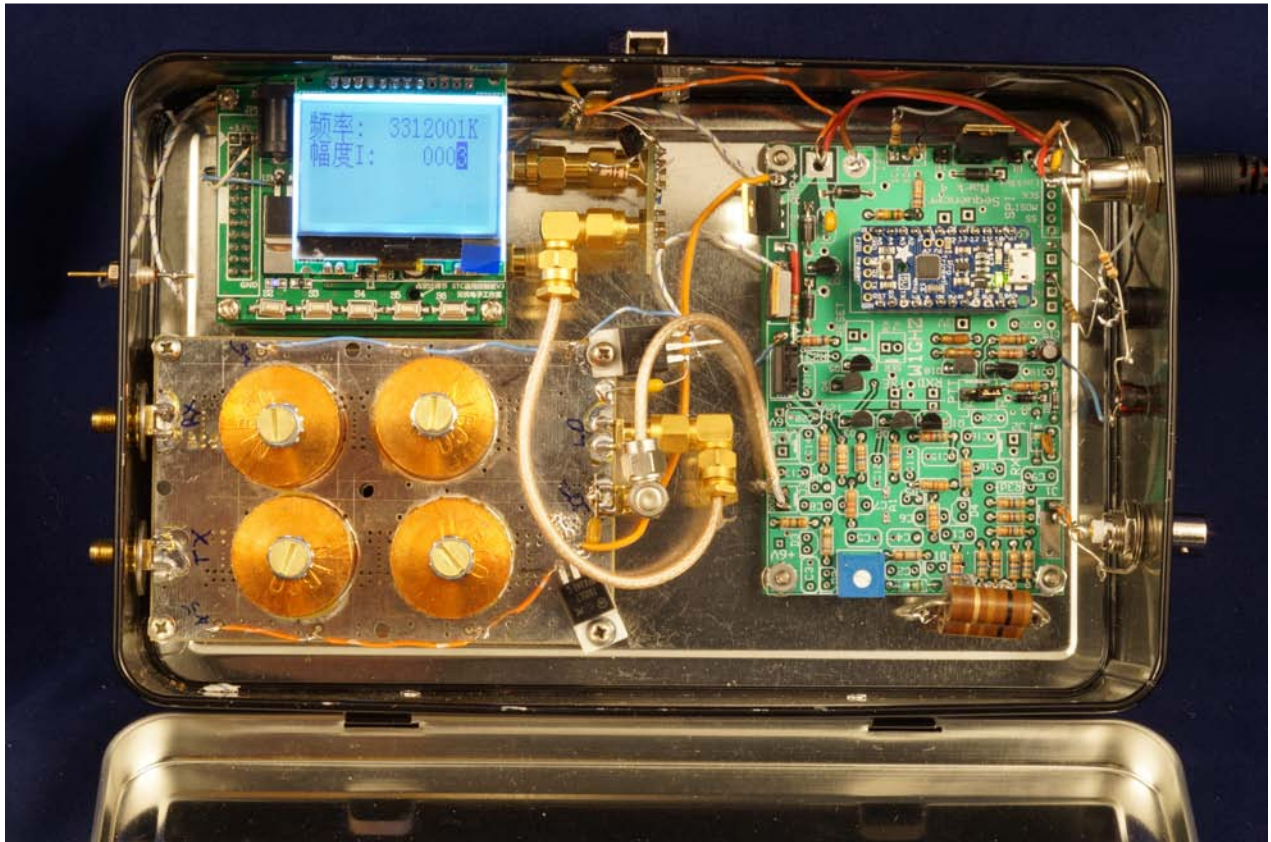
Figure 1- Simple transverter for 3456 MHz with Mark 4 Sequencer at the right
