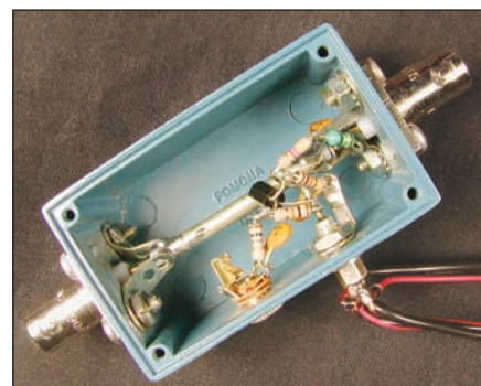
Figure 5 — A view of the dead-bug construction techniques used to build the Bias-tee.
