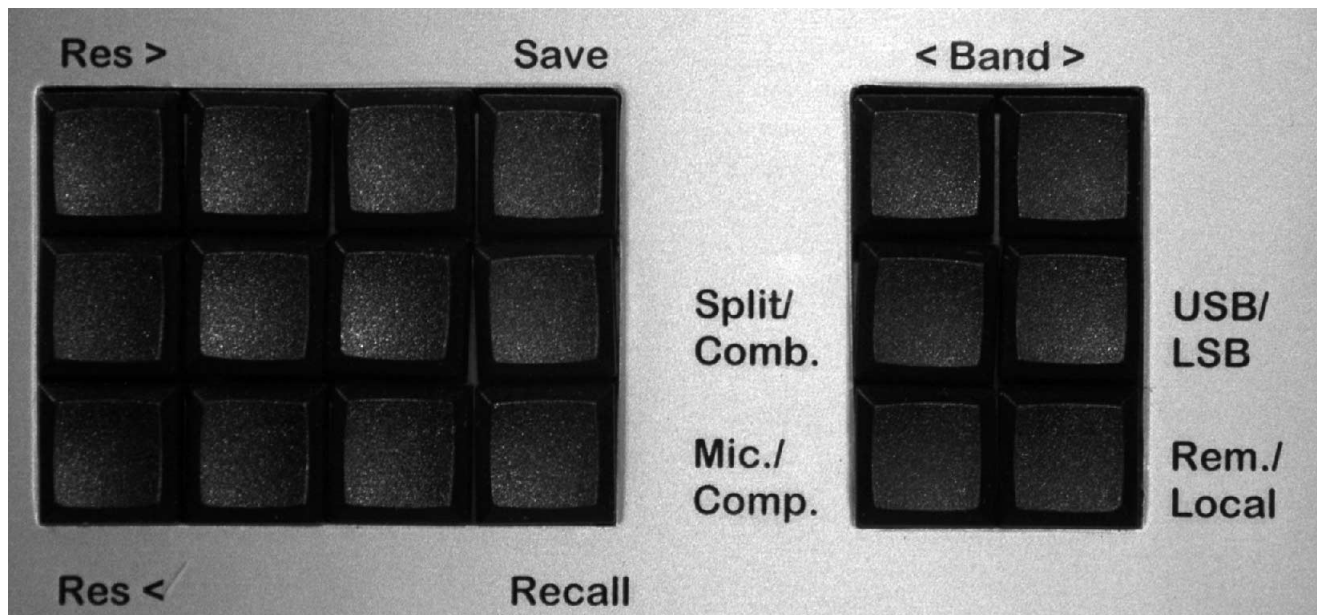
Figure 13 — The keyboard layout and key functionality with present software version. The main tuning functionality is controlled by the optically encoded main tuning knob when in Split mode
