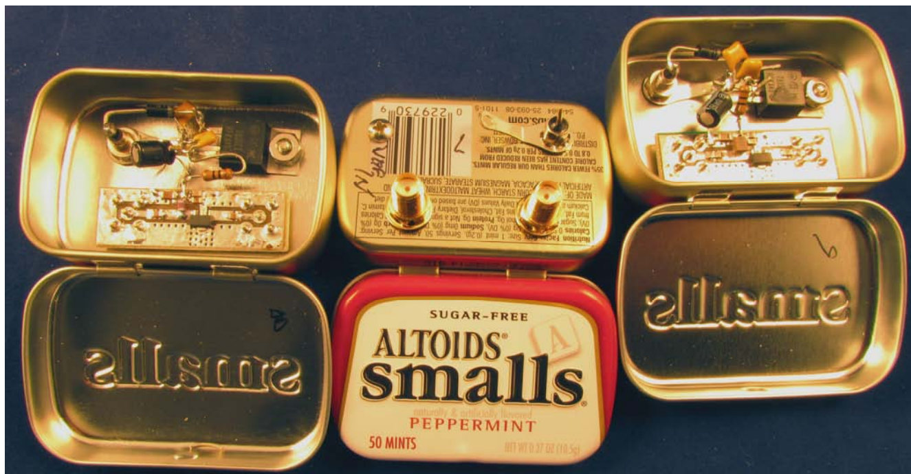
Figure 1- MMIC preamps in Altoids tins
