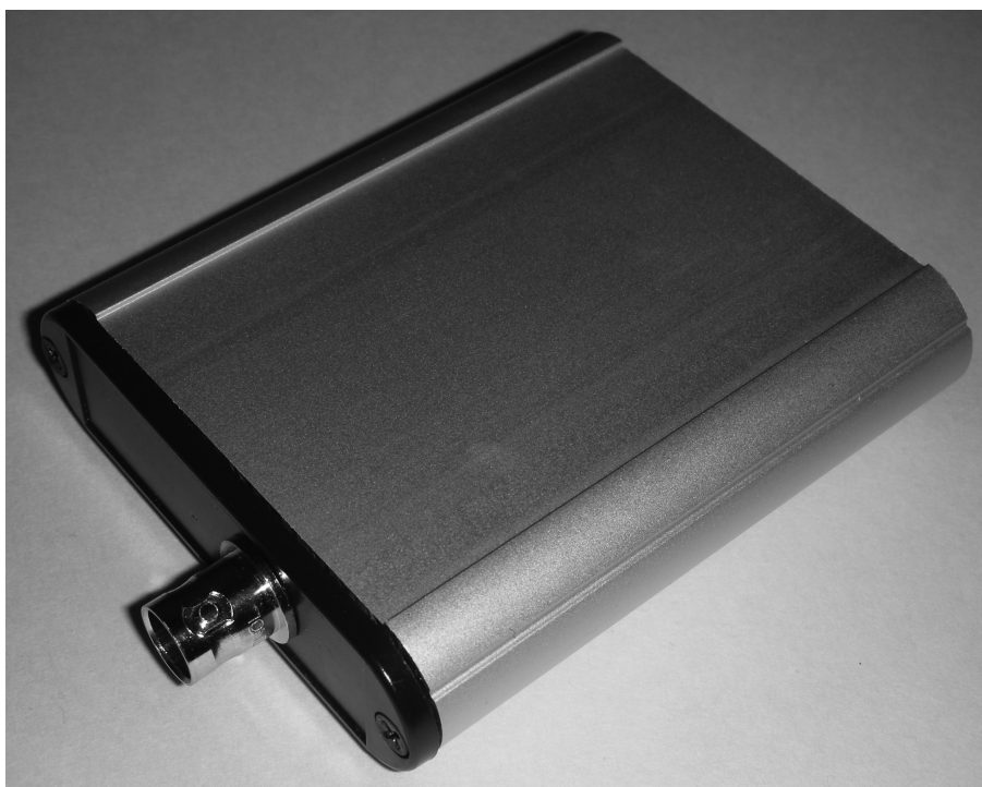
Figure 6 — The Simple SDR receiver board will fit inside a Hammond Manufacturing model 1455B802 enclosure if a chassis-mount BNC connector is used instead of the on-board connector.
