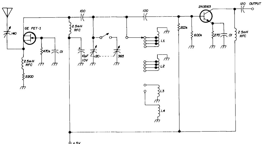
L1      31 turns no. 18 airwound, 5/8" diameter, 1-7/8" long, (B&W 3007) tapped at 2, 11 and 27 turns (tunes 4-40 MHz)
