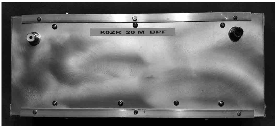
Figure 14 — The completed 20 m band pass filter. [Jeff Crawford, K0ZR, photo]
