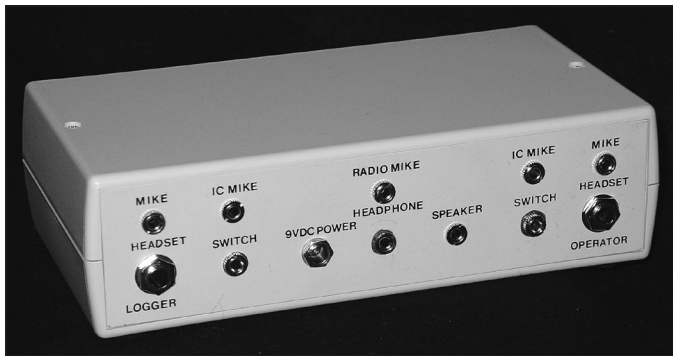
Figure 65 — Rear view of the audio interface box. Operator jacks are on the right, logger on the left. Connections to the radio are in the center.
