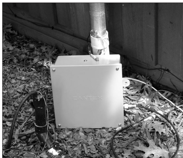
Figure 21 — The switchable matching unit mounted at the base of the author's 43-ft vertical.
