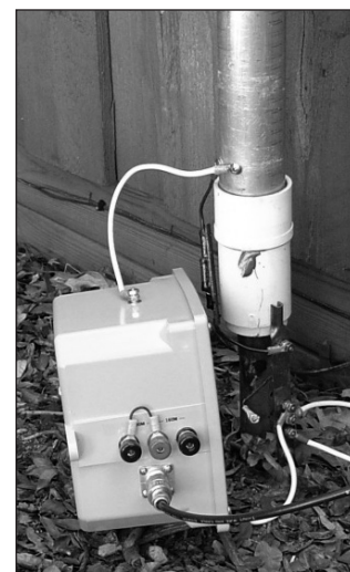
Figure 16 — The finished matching unit at the base of the author's 43-ft antenna (strapped for 80 meter operation).
