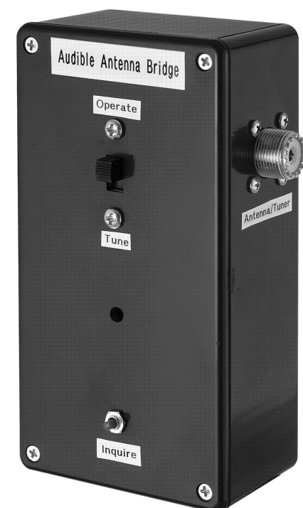
Figure 31 — Front view of the audible antenna bridge.
