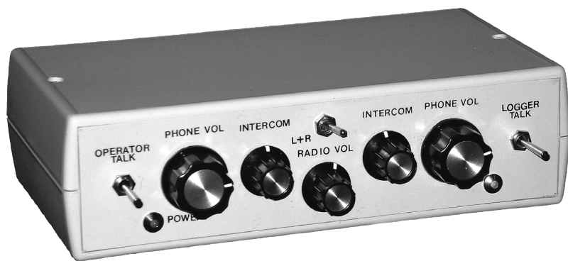
Figure 63 — Front view of the audio interface box. Operator controls are on the left and logger controls are on the right.
