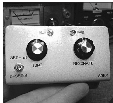
Figure 1 — The Z-Match Tuner handles 100 W and can be used from 80 through 10 meters.
