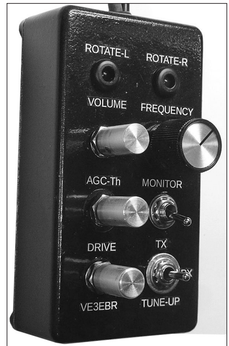
Figure 56 — The SDR Knob Box replaces software controls such as click boxes and sliders with physical knobs and switches read by an Arduino microcontroller and then relays the appropriate commands to an SDR transceiver.
