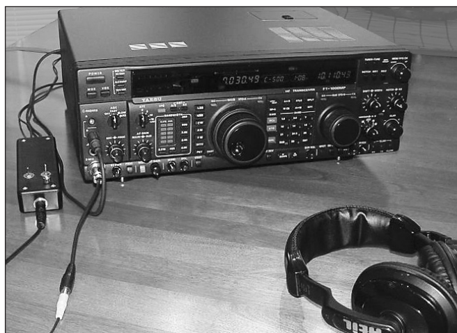
Figure 62 — The AIE takes up little desk space. It plugs inline between the transceiver and headphones and requires 13.6 V dc. In the author's shack, the unit is powered from a transceiver accessory jack and is always switched on.
