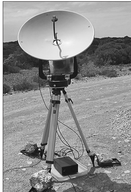
Figure 68 — The portable EME-capable 10 GHz station of VK7MO, set up at roadside in the Australian outback.
