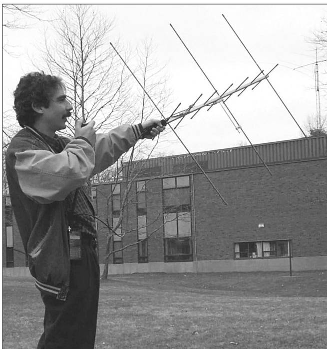
Figure 18 — Joe Bottiglieri, AA1GW, uses a dual-band Yagi to work a low-Earth orbiting FM repeater satellite with a handheld transceiver.
