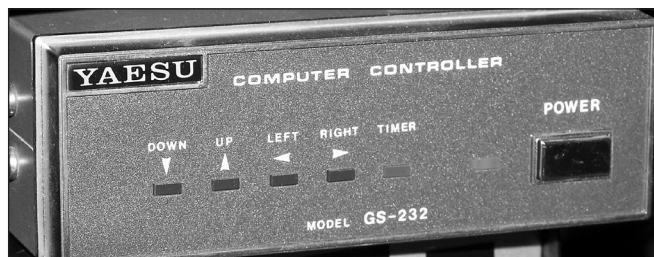
Figure 30 — The Yaesu GS-232 allows your computer and satellite tracking software to automatically control the movements of compatible azimuth/elevation antenna rotators.
