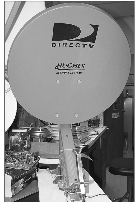
Figure 24 — This is a good example of an offset-fed dish. Note the feed source at the bottom edge of the photo, pointing into the center of the parabola. Also note that this is a DirectTV satellite TV antenna that has been “repurposed” for amateur radio satellites!
