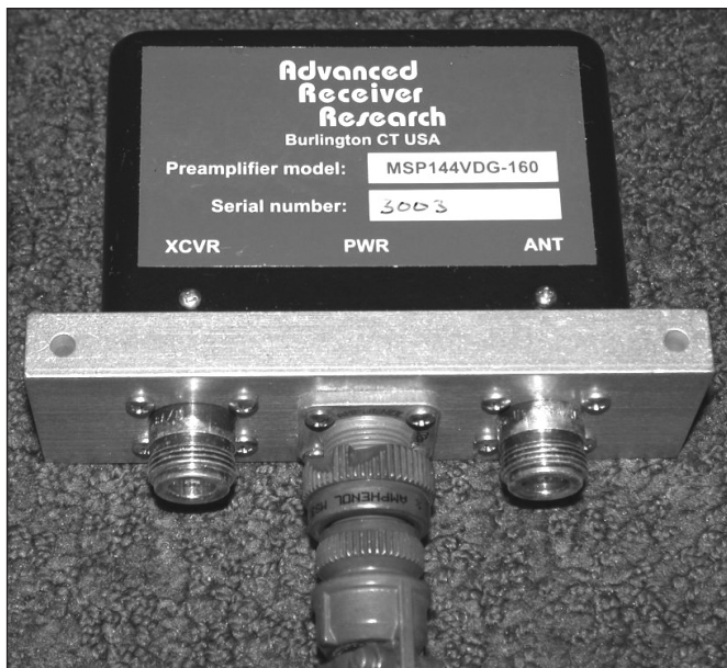
Figure 31 — This receive preamplifier by Advanced Receiver Research gives signals a substantial boost before they travel down the coaxial cable to your radio.
