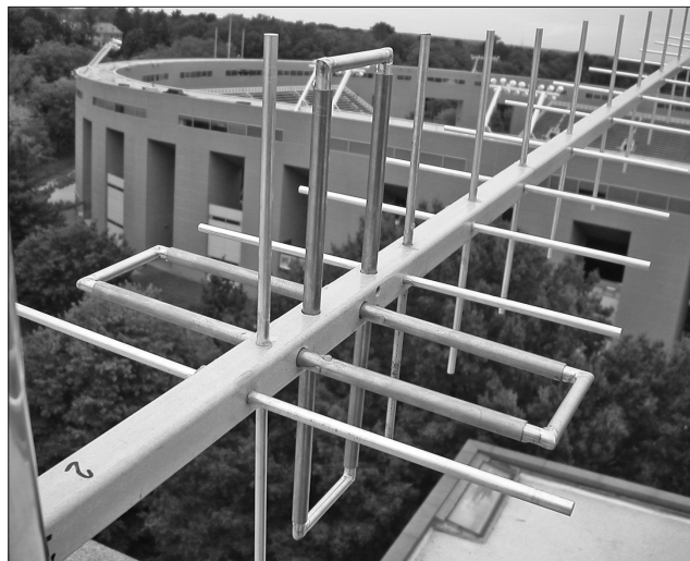
Figure 72 — Dual-polarization EME array at W2PU. At the left, shows the four 15-element, rear-mounted Yagis. Boom length is 3.5 m, and stacking distance is 1.2 m in each direction. The right photo is a close-up showing some details around the driven loops.
