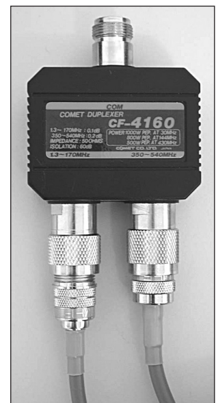
Figure 19 — A diplexer made by the Comet Corporation. Diplexers can be used to separate or combine signals on different bands.
