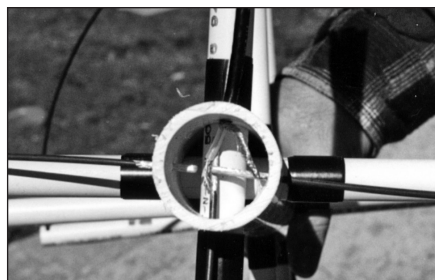
Figure 58 — An end-on view of the top of the QHA prior to soldering the loops and installing the PVC cap.
