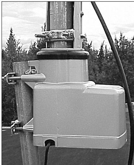
Figure 26 — A basic antenna rotator; the light-duty variety used to turn TV antennas. The wire exiting the bottom of the rotator housing is the multiconductor cable responsible for power and control.
