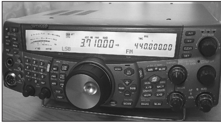
Figure 40 — The Kenwood TS-2000 offers full HF coverage along with VHF/UHF full-duplex satellite capability.
