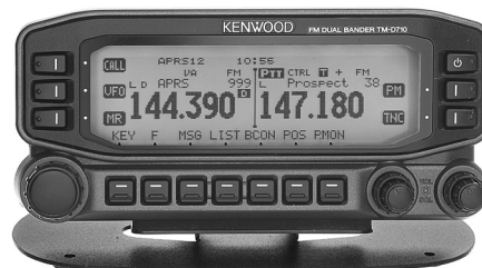
Figure 37 — The Kenwood TM-D710 is a dual-band FM transceiver with a built-in packet radio Terminal Node Controller (TNC) for digital communication.
